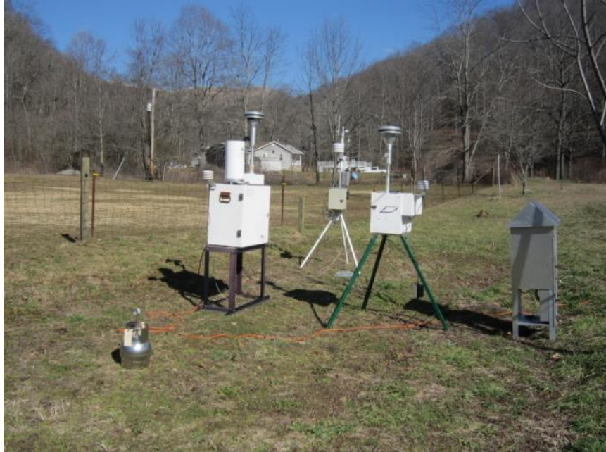
Figure 28. Photograph of particle sampling and meteorological monitoring equipment at residence.
