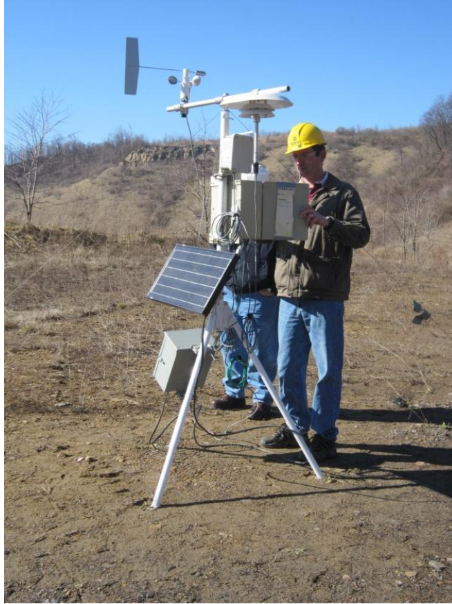
Figure 31. Meteorological monitoring equipment at mine site.
