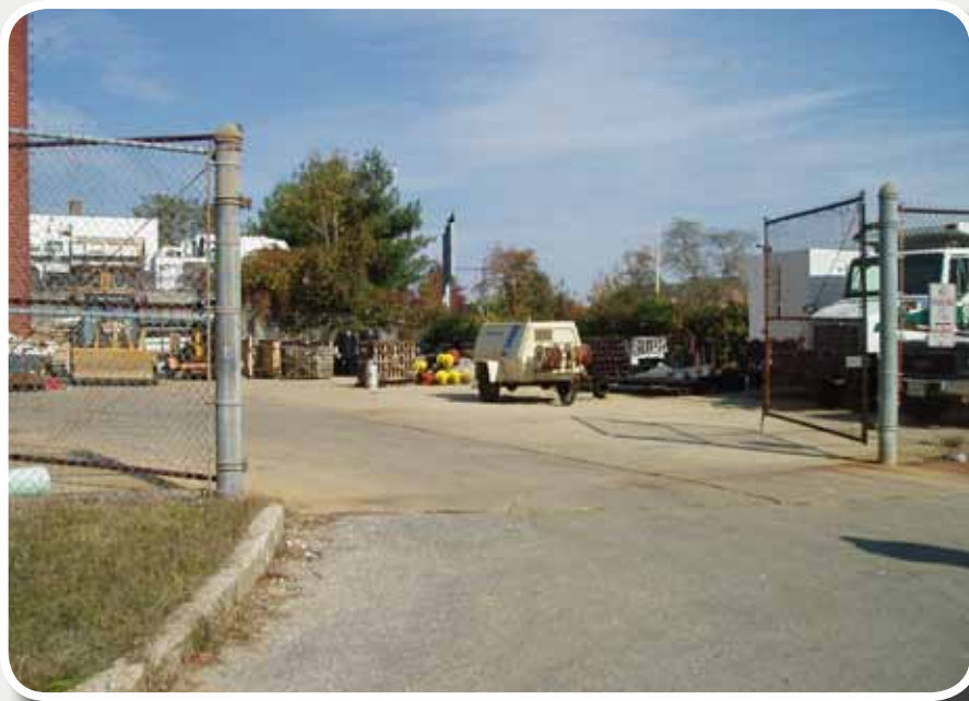
Figure 2.7. Public works yards are one type of stormwater hotspot due to the high number of potential polluting materials stored outside (Source: Center for Watershed Protection)
