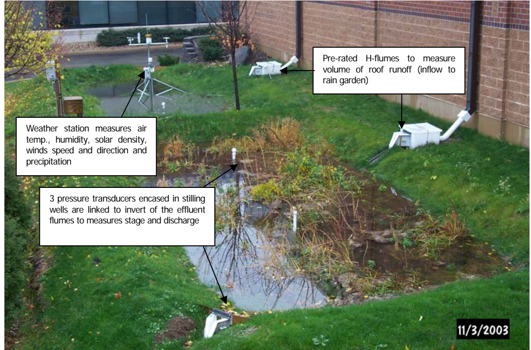
Figure 2. Example monitoring set-up to estimate a water mass balance for a paired rain garden study. (Courtesy of W. Selbig, USGS-WI)
