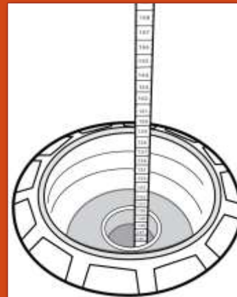
Manual tank gauging
