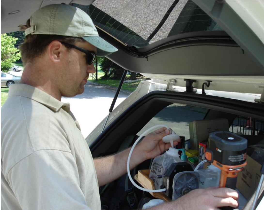
Figure 3-11. Example of Peristaltic Pump/Drill Apparatus for Sample Filtration being used under the tailgate of a vehicle.
