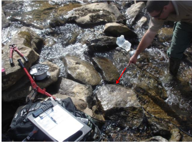
Figure 13-15. Picture of sonde concealed by large substrate.
