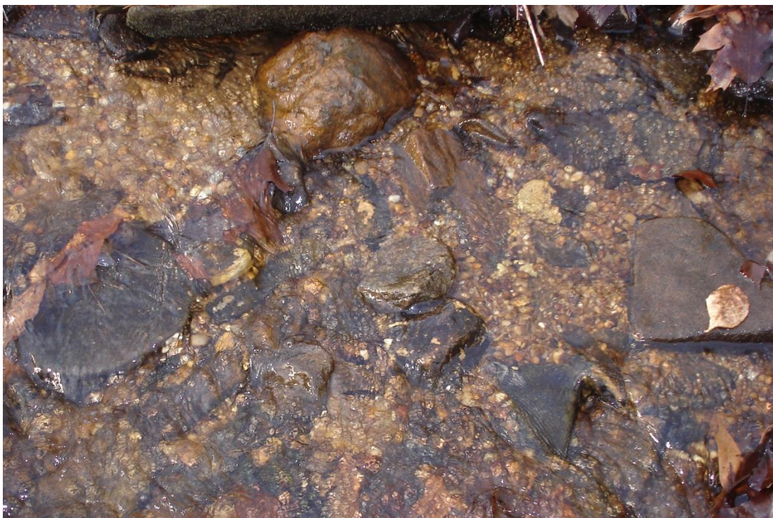
Figure 2-31. Example of cobble that is partially embedded.
