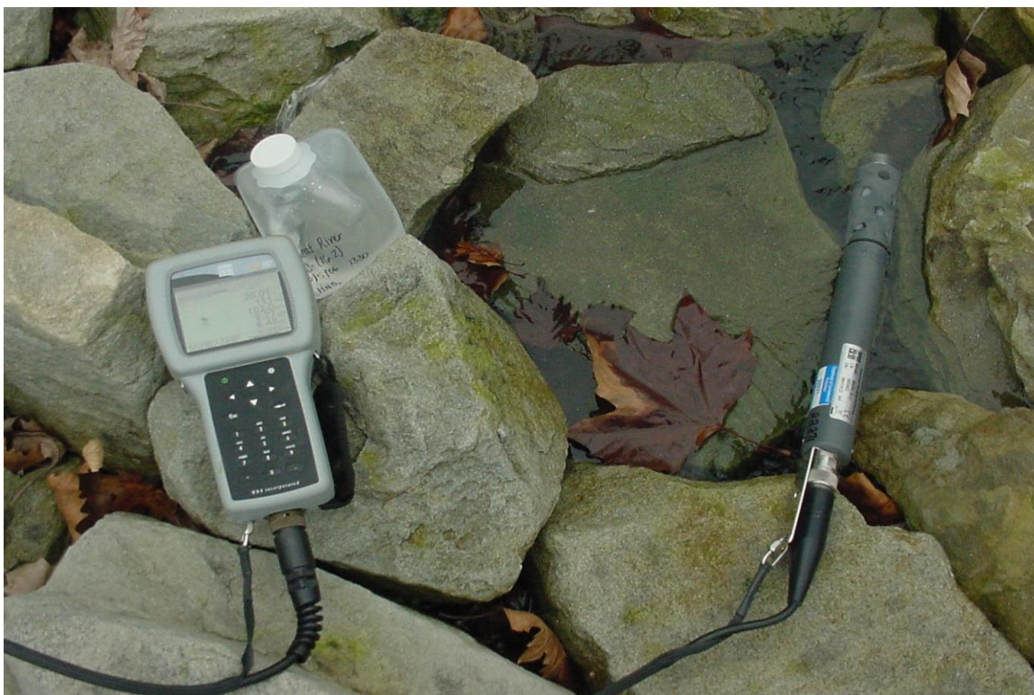
Figure 3-1. Example of a YSI 660 XL Sonde (right) and a 650 MDS Display Unit (left).
