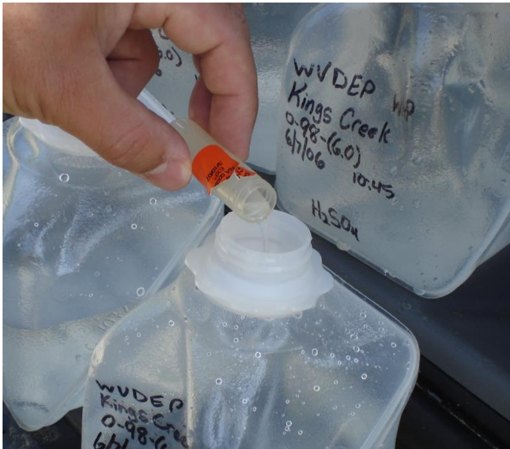
Figure 3-12. Example of sample being preserved with Nitric Acid.
