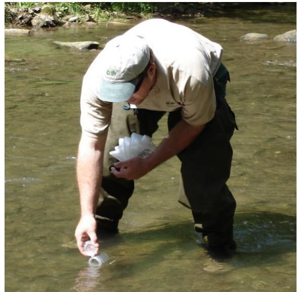
Figure 3-9. Example of a Fecal Sample being taken from a stream.
