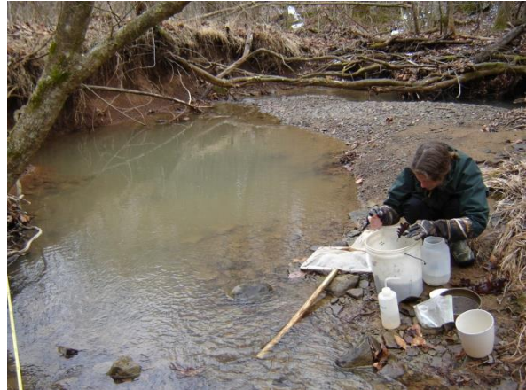
Figure 5-8. Photograph of Biologist inspecting benthic sample and removing rough material (rocks, sticks, and leaves)
