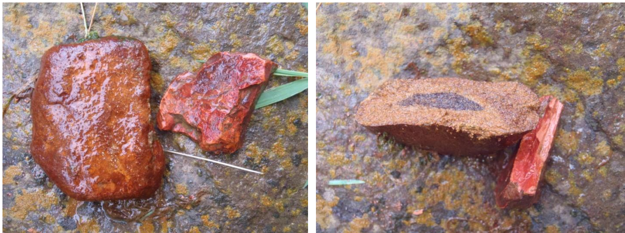
Figure 2-13. Left: An iron coated rock on left and a piece of red dog on right. Right: A cross section of the same rocks (iron coated rock on left and a piece of red dog on right).
