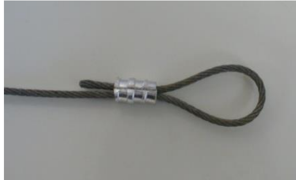
Figure 13-5. Picture of typical anchor loop.
