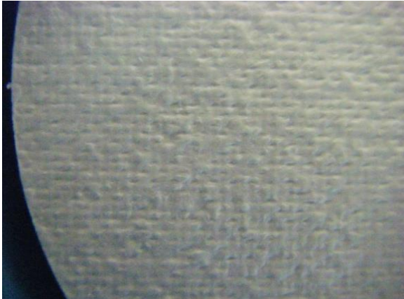
Figure 9-6. Photo of the gridded pattern of GF/F filter. This side placed down when filtering Golden Algae sample.
