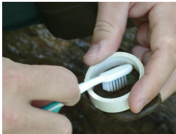
Figure 7-2. Toothbrush being used to scrub remaining algae and periphyton from upper surface of rock.
