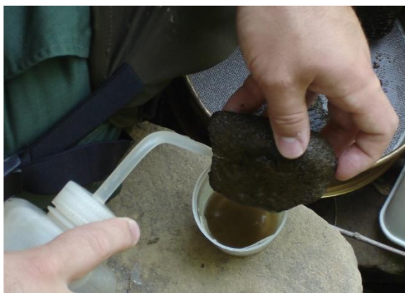
Figure 7-3. Loosened algae and periphyton being rinsed into the sample jar.
