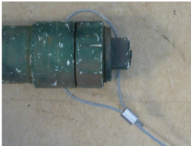
Figure 13-6. Picture of anchor cable looped directly thru the PVC sonde case.
