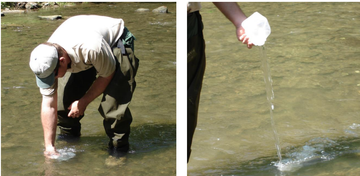
Figure 3-10. Example of Cubitainer being filled and emptied (i.e., rinsed with stream water).
