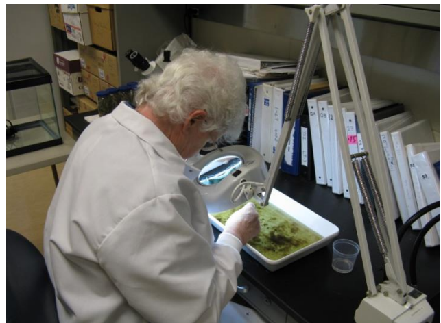
Figure 5-15. Photograph of Biologist sorting a benthic sample under an illuminated magnifier. Note the enamel pan filled with some water and the temporary sample container.
