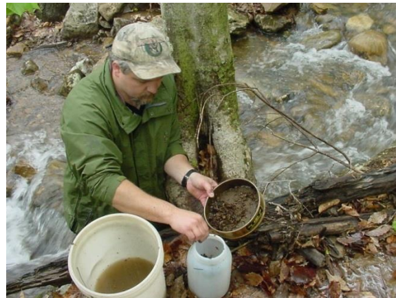
Figure 5-11. Photograph of Biologist inspecting transferring the soft, organic material (e.g., shredded leaves and benthic organisms) to the sample jar.
