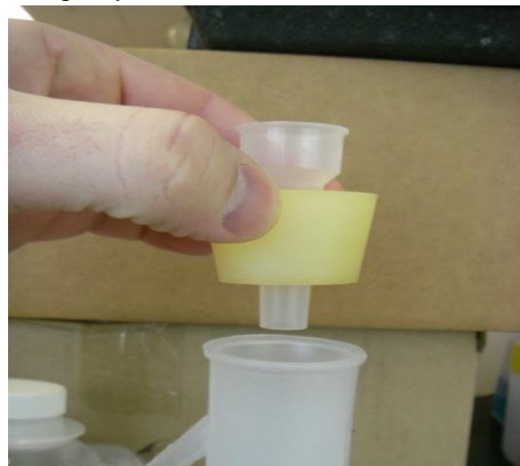
Figure 9-3. Photo of the insertion of rubber stopper into flask with plastic funnel already inserted through rubber stopper.
