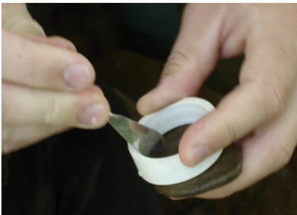
Figure 7-1. Microspatula being used to scrape algae and periphyton from upper surface of
