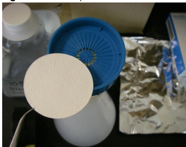
Figure 9-5. Photo of the GF/F filter being placed on top of support screen with forceps.
