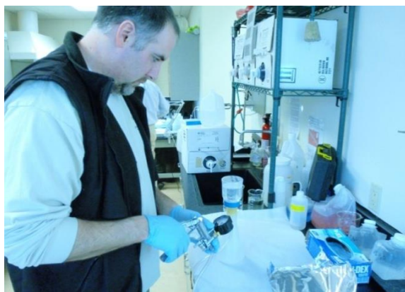
Figure 9-8. Photo of monitoring the pump pressure while filtering sample – keep the pressure under 5 psi.
