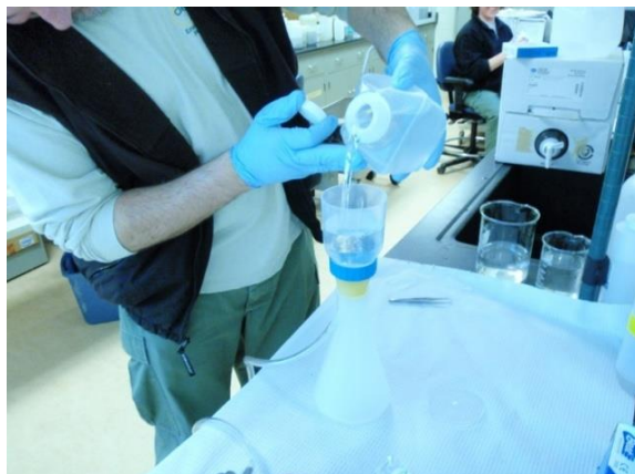
Figure 9-7. Photo of the pouring of a 250 mL sample into filter cup.
