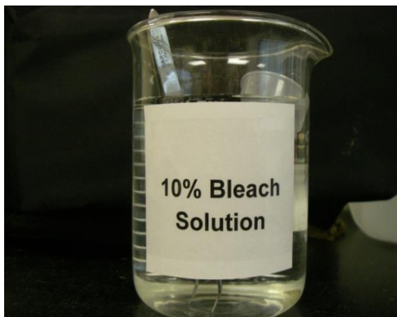
Figure 9-10. Photo of Forceps and small plastic funnel soaking in 10% bleach solution for 1 minute.
