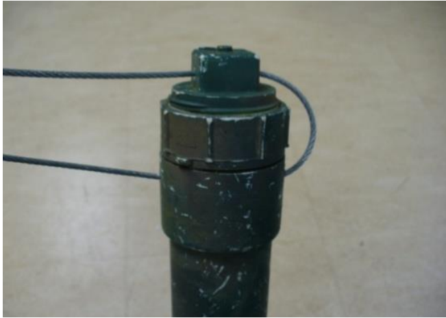
Figure 13-8. Picture of cable threaded thru PVC sonde case and then looped thru screw cap.
