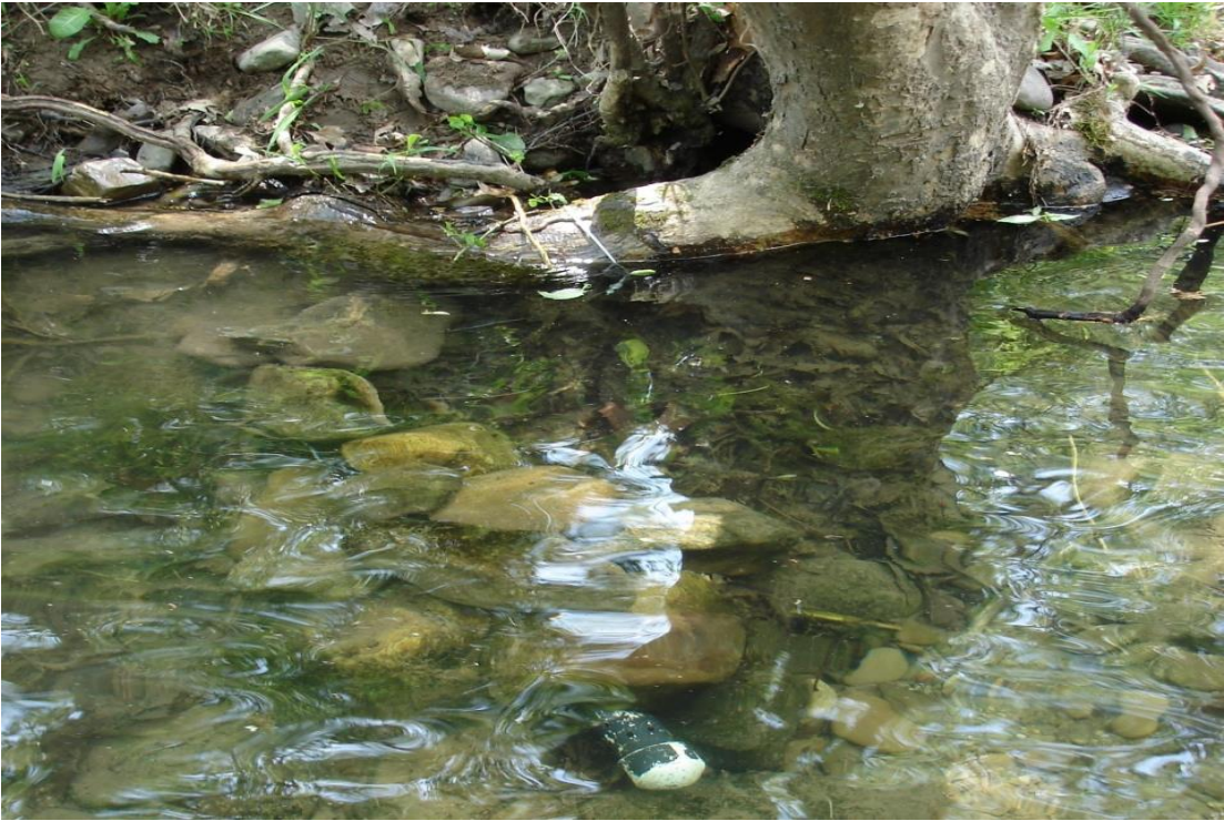
Figure 13-21. Picture of sonde concealed by cobble in pool created by rootwad.
