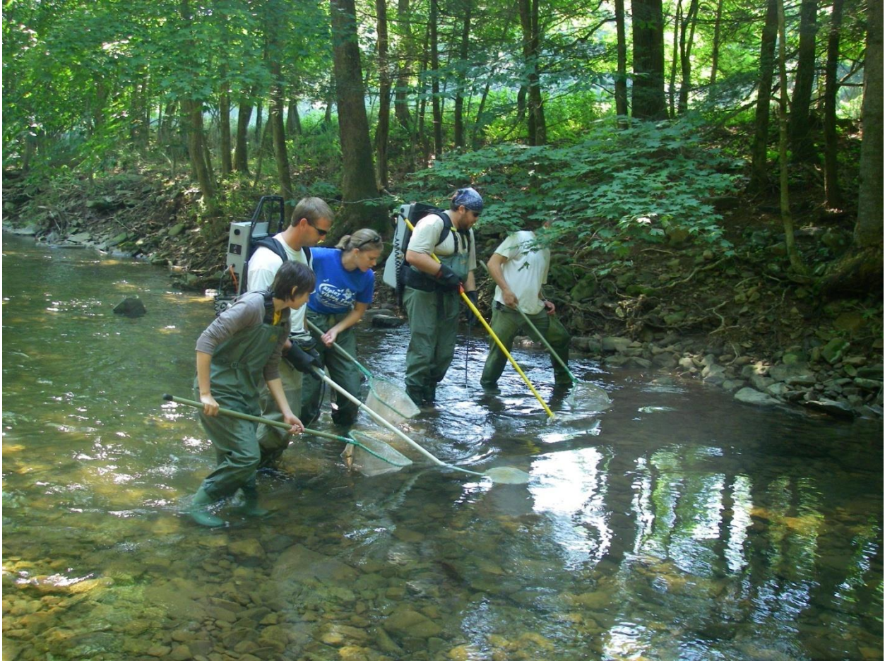
Figure 6-3. An electrofishing crew consisting of two backpack shockers (electrofishers) and three netters.
