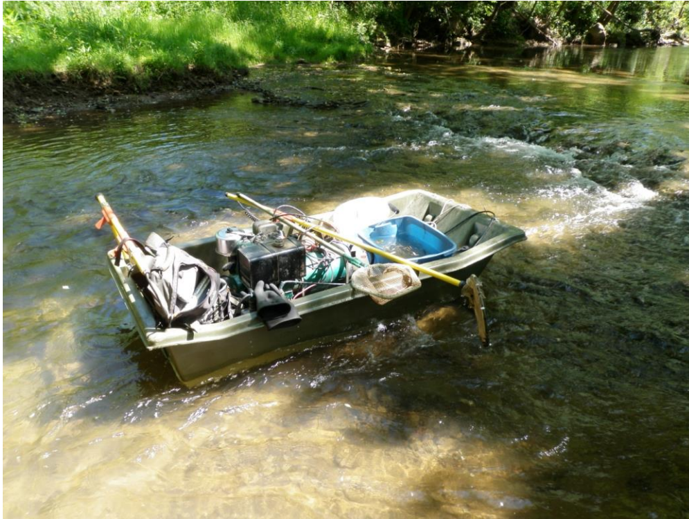
Figure 6-5. Tow barge with generator, live well, and shocking wand.
