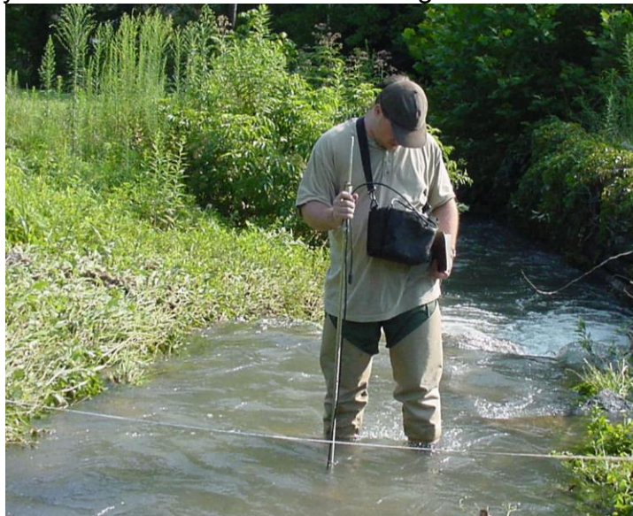
Figure 4-5. Example of taking flow measurements at a transect.
