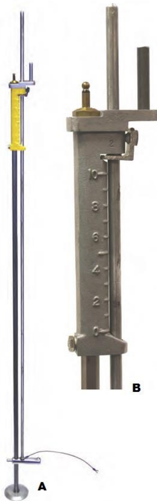
Figure 4-4. A) Top-Setting Wading Rod and B) Close-up of handle or Top-Setting Wading Rod.
