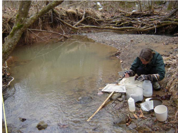
Figure 14. Photograph of Biologist inspecting benthic sample and removing rough material (rocks, sticks, and leaves)
