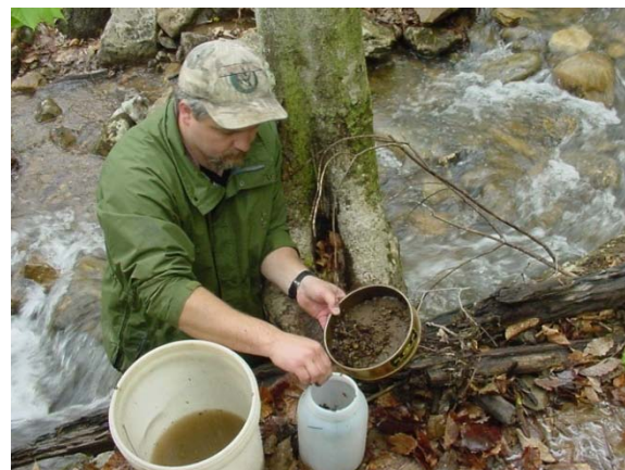
Figure 17. Photograph of Biologist inspecting transferring the soft, organic material (e.g., shredded leaves and benthic organisms) to the sample jar.
