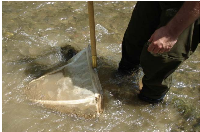
Figure 11. Photograph of the Kicking process in front of the net.
