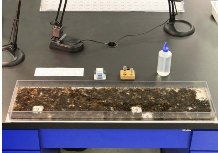
Figure 20. Photograph of a Gridded Sorting Tray with 5 grids randomly removed. Note that the sequence of numbers on the bottom of the tray known by referencing a piece of paper that has the locations of each grid mapped out.
