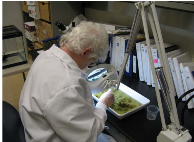
Figure 21. Photograph of Biologist sorting a benthic sample under an illuminated magnifier. Note the enamel pan filled with some water and the temporary sample container.
