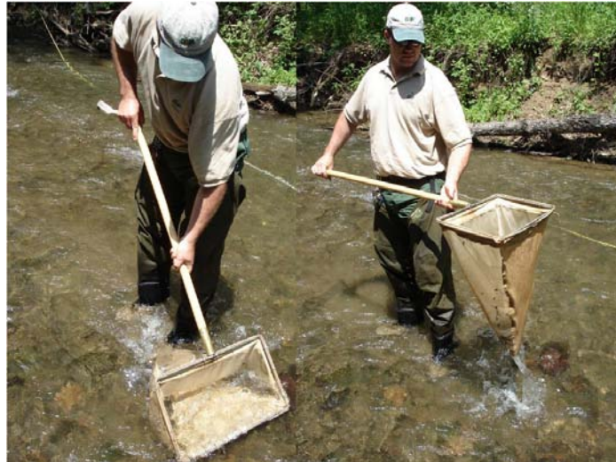
Figure 12. Photographs showing the removal of the net from the water with an upstream motion.
