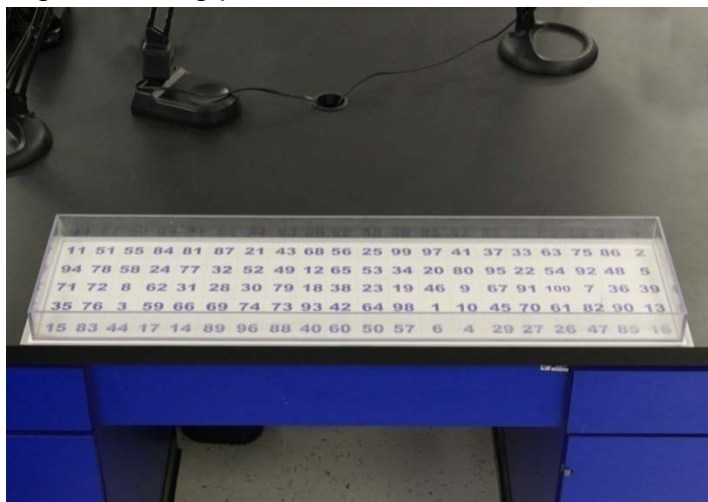
Figure 18. Photograph of a Home-Made Gridded Sorting Tray featuring a random number matrix on the bottom.
