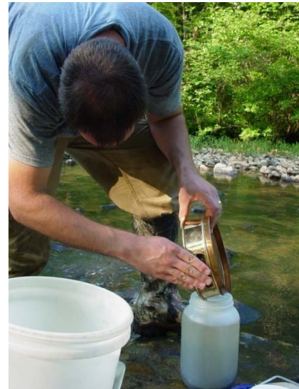
Figure 16. Photograph of Biologist transferring the hard, inorganic material (e.g., fine gravel, sand, and silt) to a sample jar ½ filled with alcohol.
