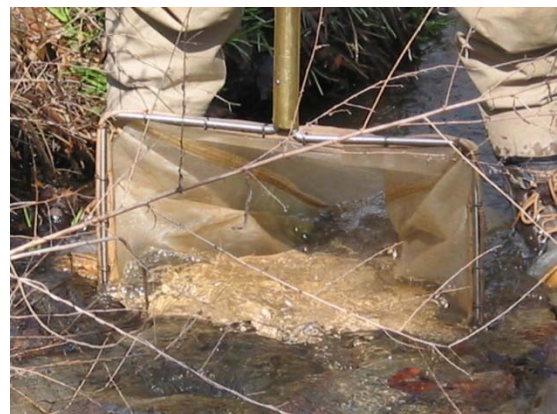
Figure 9. Photo of Rectangular Frame Dip Net being placed on stream bottom
