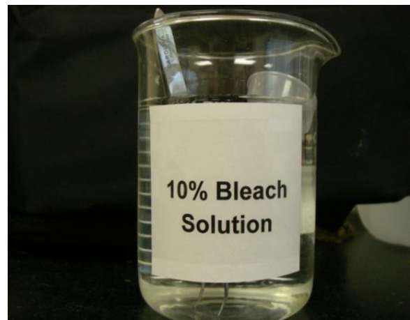
Figure 9-10. Photo of Forceps and small plastic funnel soaking in 10% bleach solution for 1 minute.
