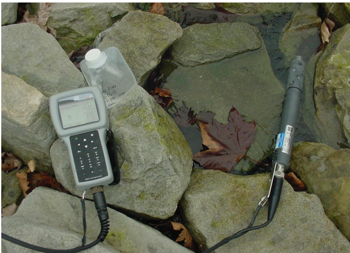
Figure 3-1. Example of a YSI 660 XL Sonde (right) and a 650 MDS Display Unit (left).
