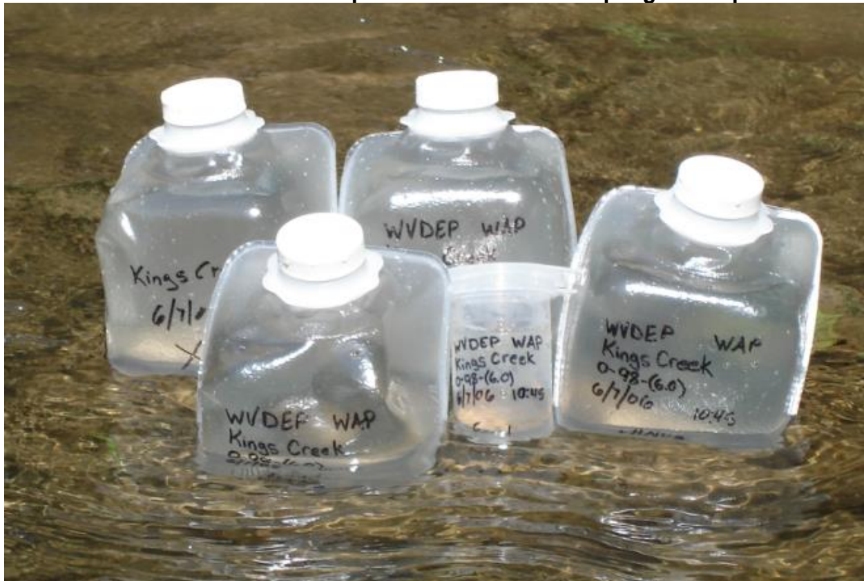
Figure 3-9. Example of Sample Containers Labeled with sample information.
