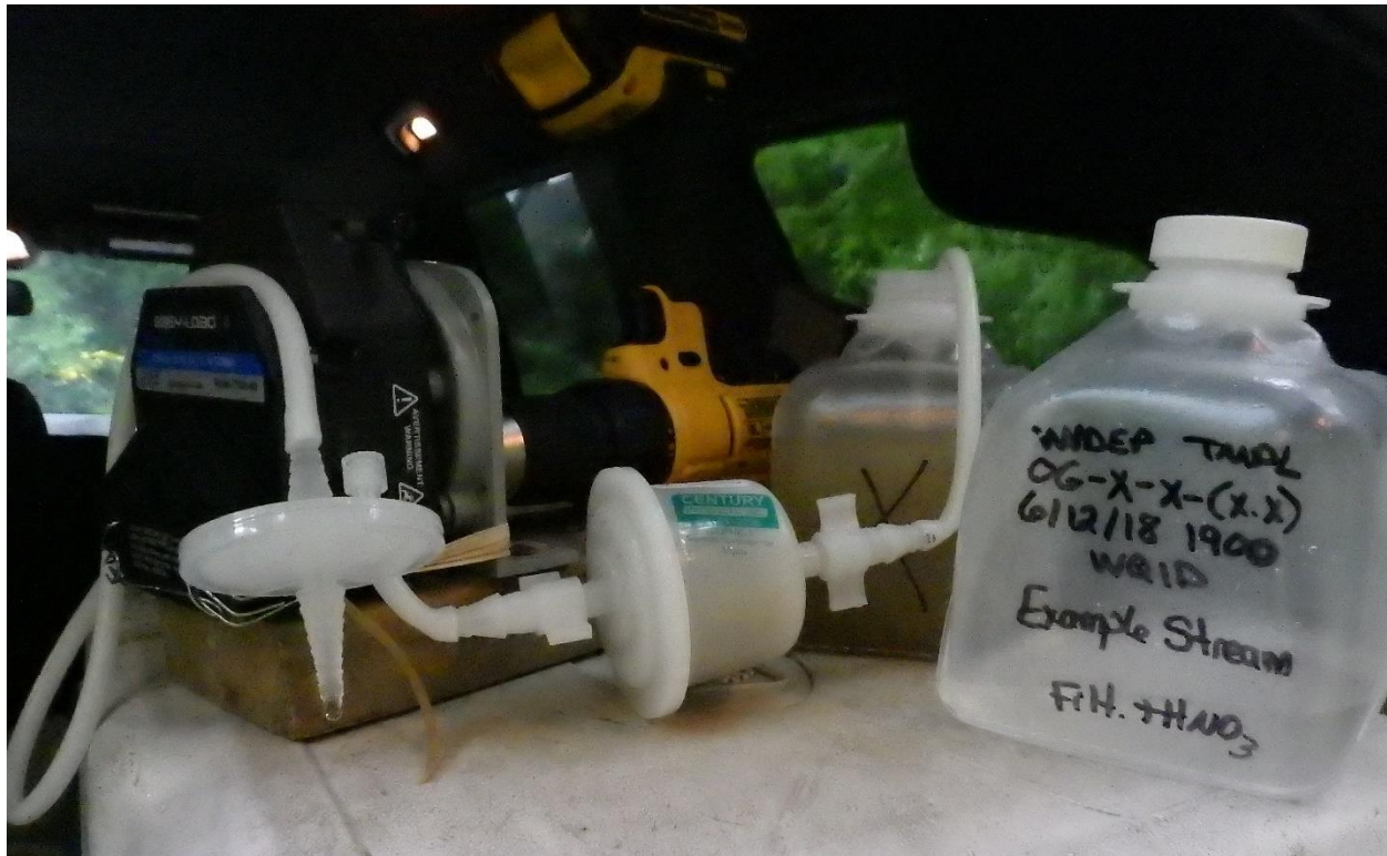
Figure 3-14. Example of Filtration Setup with a Cartridge and Disk Filterer
