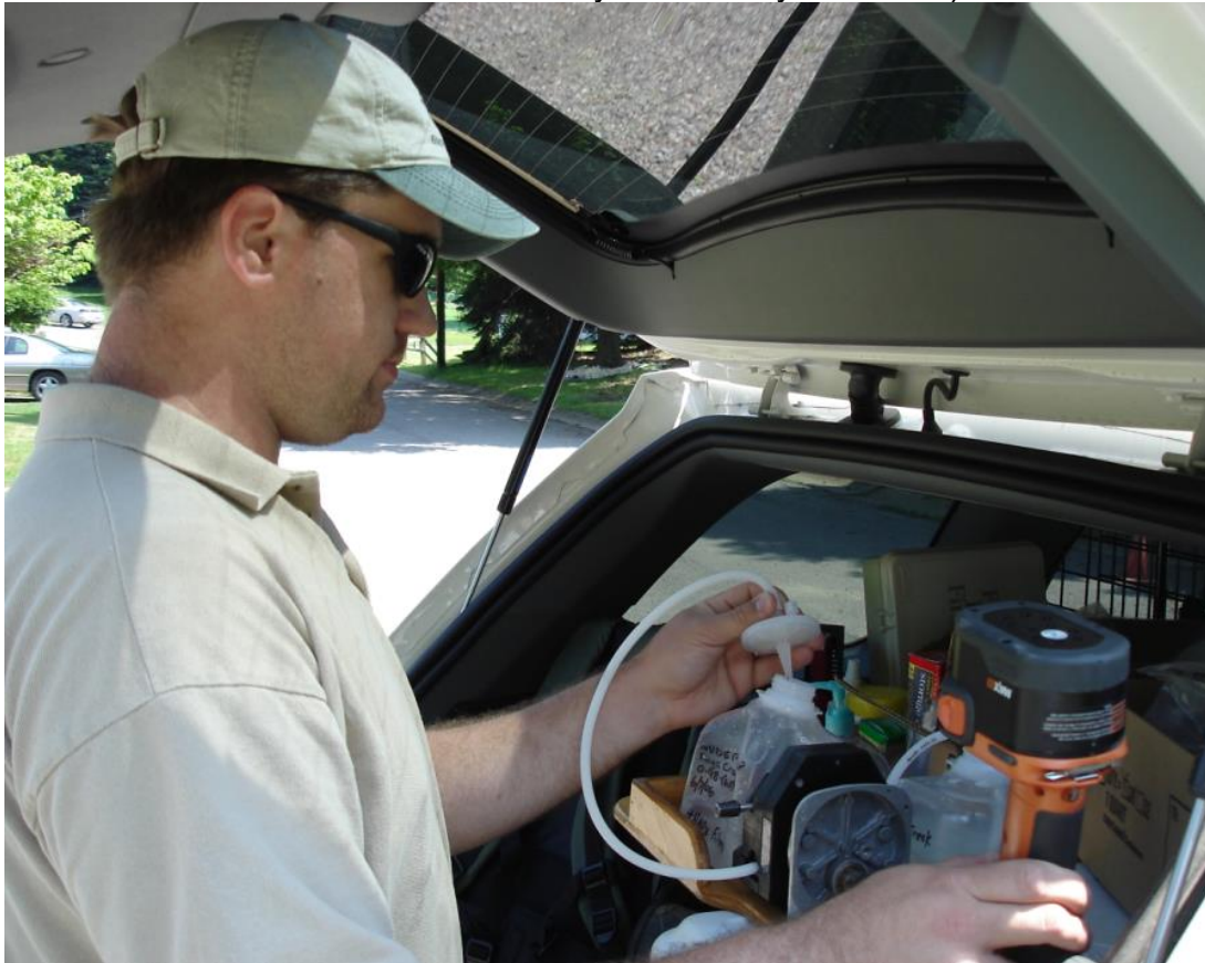
Figure 3-12. Example of Peristaltic Pump/Drill Apparatus for Sample Filtration being used under the tailgate of a vehicle.
