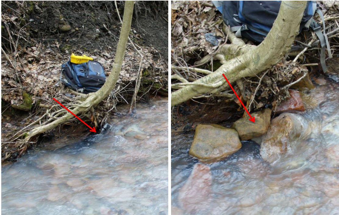
Figure 13-20. Picture of sonde before (left) and after (right close-up) concealment with cobble. Arrow points to sonde placed in stream channel.
