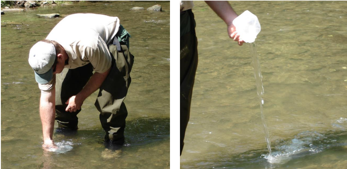
Figure 3-11. Example of Cubitainer being filled and emptied (i.e., rinsed with stream water).
