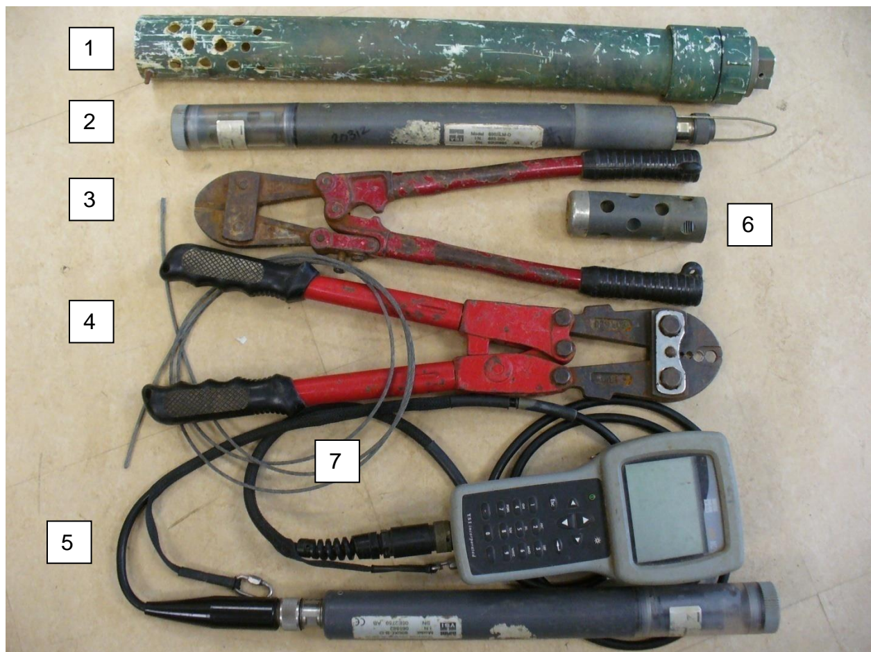
Figure 13-1. Items Required for Deploying the Continuous Monitor
