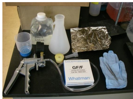
Figure 9-1. Photo of the materials used to filter a Golden Algae sample.
