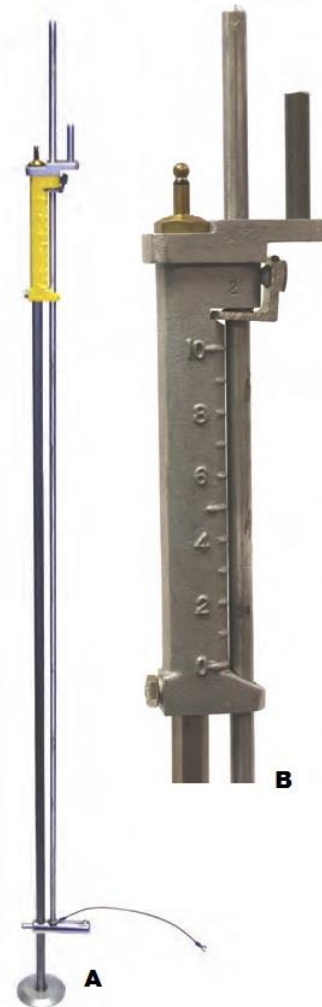
Figure 4-2. A) Top-Setting Wading Rod and B) Close-up of handle or Top-Setting Wading Rod.
