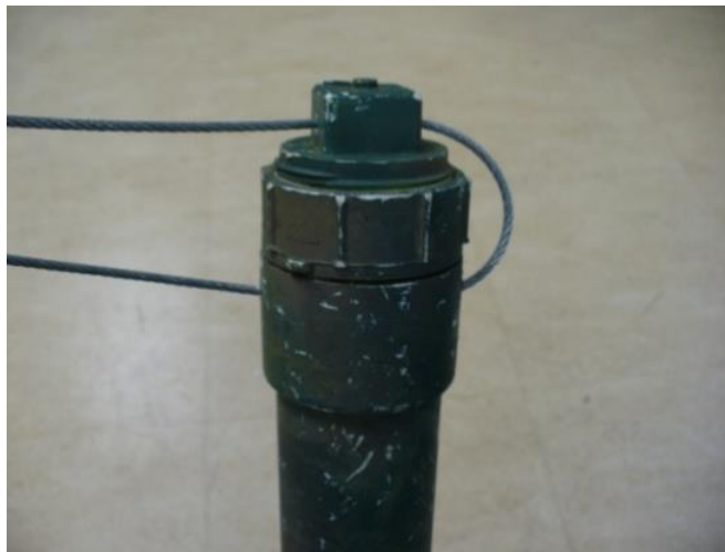
Figure 13-8. Picture of cable threaded thru PVC sonde case and then looped thru screw cap.
