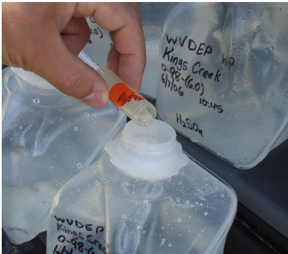
Figure 3-15. Example of sample being preserved with Nitric Acid.
