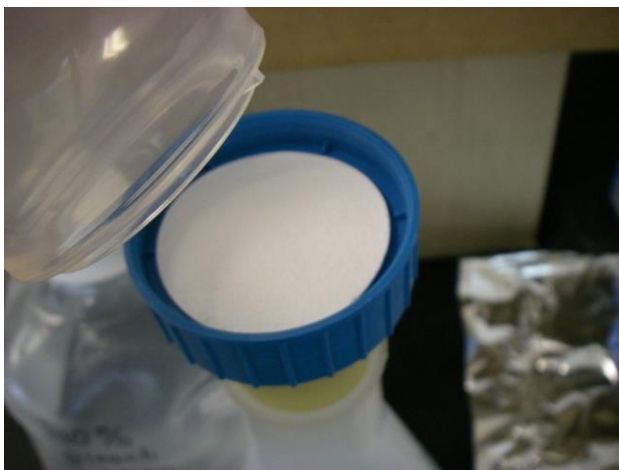
Figure 9-4. Photo of cup being removed to access the prepackaged filter for removal.
