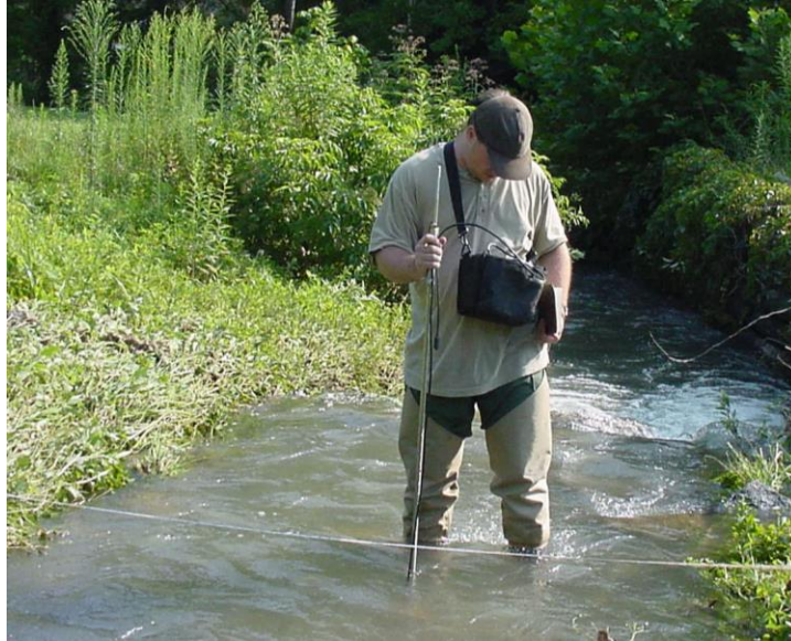
Figure 4-4. Example of taking Flow Measurements at a Transect.
