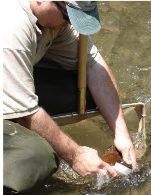
Figure 5-4. Photograph of the Brushing process in front of the net.
