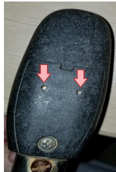
Figure 4-7. Location of Depth Sensors on OTT MF Pro
