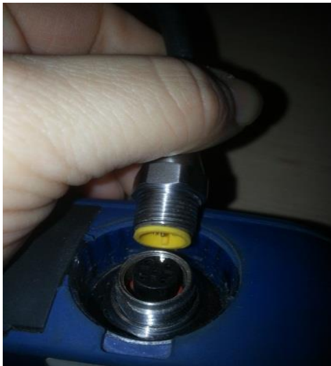
Figure 4-12. OTT MF Pro Cable attachment to Hand Set
