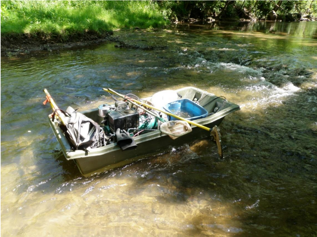
Figure 6-6. Tow barge with generator, live well, and shocking wand.
