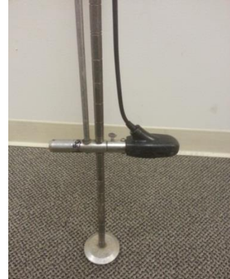
Figure 4-11. OTT MF Pro Sensor attached to end of wading rod.
