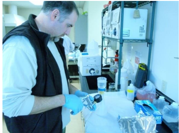
Figure 9-8. Photo of monitoring the pump pressure while filtering sample – keep the pressure under 5 psi.
