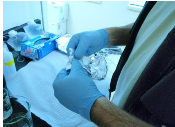
Figure 9-9. Photo of the filter disk being wrapped loosely in one 4"X4" aluminum foil square to prevent loss of algal cells via compression and smearing
