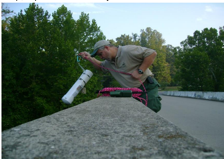
Figure 11-2. Example of PVC Sampler being used at a Bridge to Sample the Water Column
