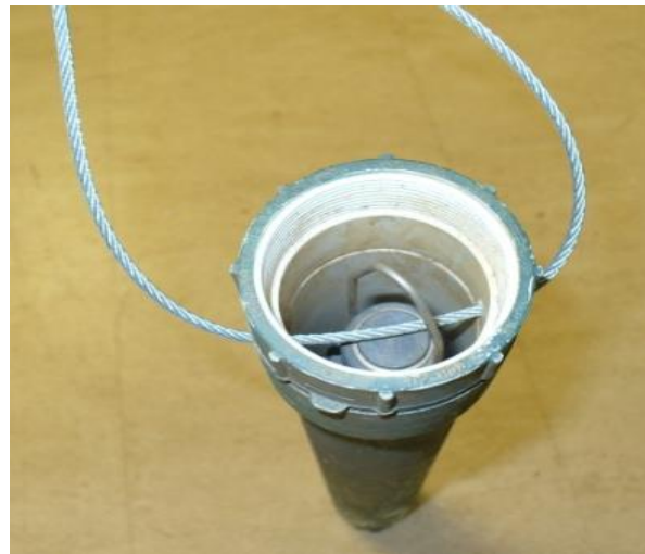
Figure 13-7. Picture of cable looped thru PVC sonde case and sonde.
