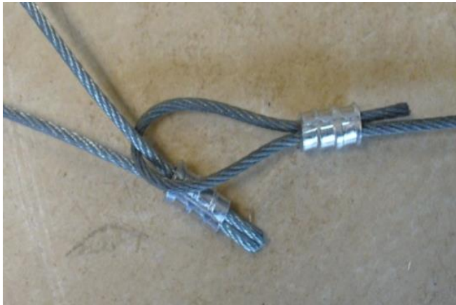
Figure 13-9. Picture of a loop used as a semi-permanent anchor interlocked with a temporary loop attached to the end of the sonde case.
