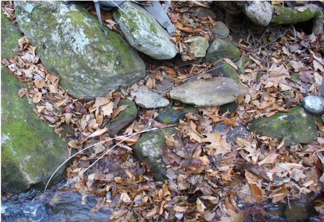
Figure 13-16. Picture of sonde anchor wire before concealment with cobble.
