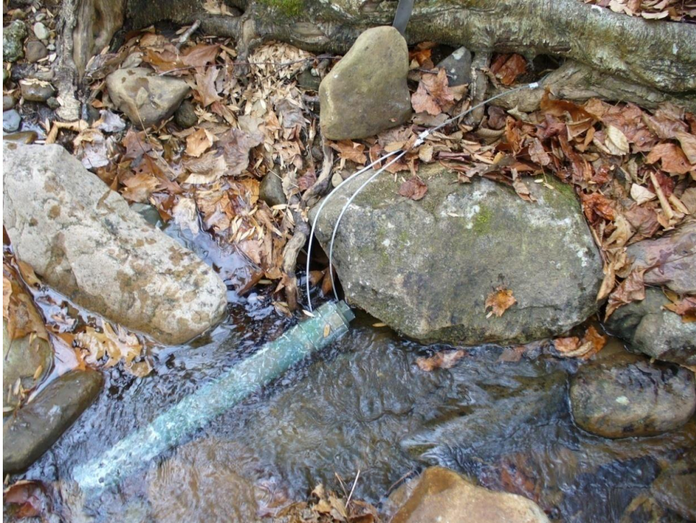
Figure 13-18. Picture of sonde anchor wire before concealment with cobble.
