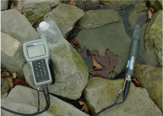
Figure 3-1. Example of a YSI 660 XL Sonde (right) and a 650 MDS Display Unit (left).
