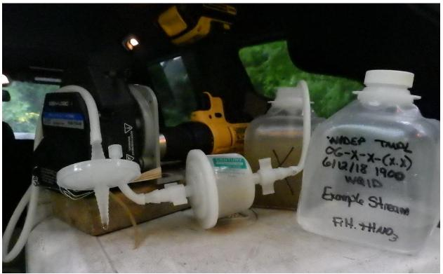
Figure 3-14. Example of Filtration Setup with a Cartidge and Disk Fileter
