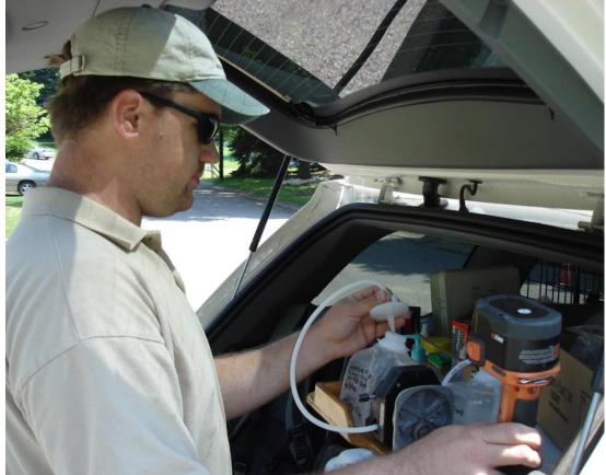
Figure 3-12. Example of Peristaltic Pump/Drill Apparatus for Sample Filtration being used under the tailgate of a vehicle.
