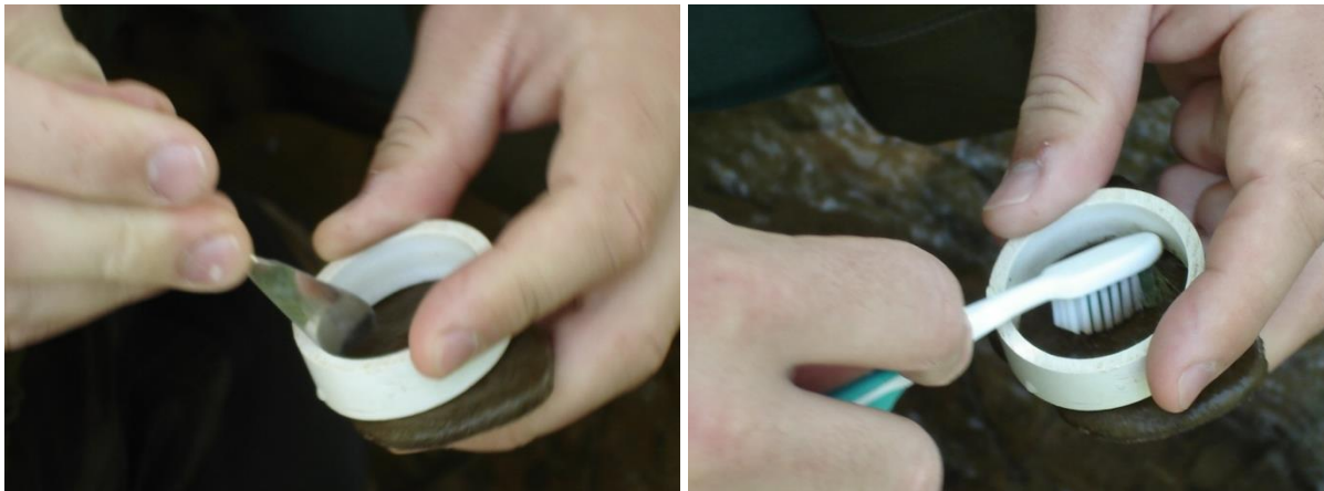
Figure 7-1. Micro spatula (left) and toothbrush (right) being used to scrape algae and periphyton from upper surface of rock.
