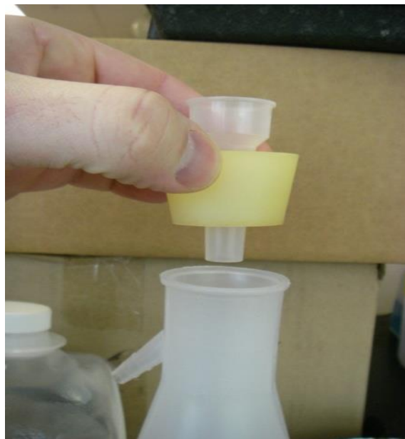
Figure 9-3. Photo of the insertion of rubber stopper into flask with plastic funnel already inserted through rubber stopper.
