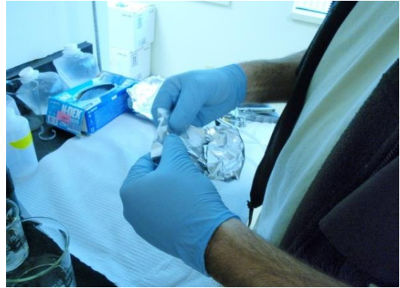
Figure 9-9. Photo of the filter disk being wrapped loosely in one 4"X4" aluminum foil square to prevent loss of algal cells via compression and smearing
