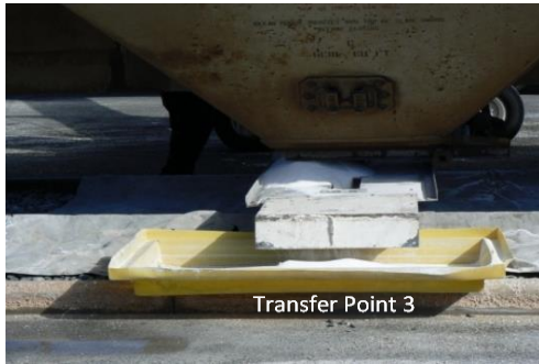
Photograph showing Transfer Point 3 (Conveyor Return to Collection Bin)
