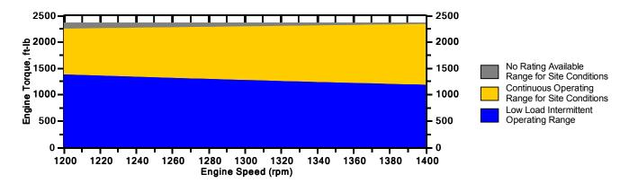
Note: At site conditions of 1200 ft and 90°F inlet air temp., constant torque can be maintained down to 1400 rpm. The minimum speed for loading at these conditions is 1200 rpm.
