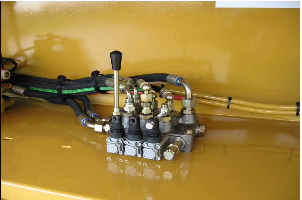
Extended main conveyor control
