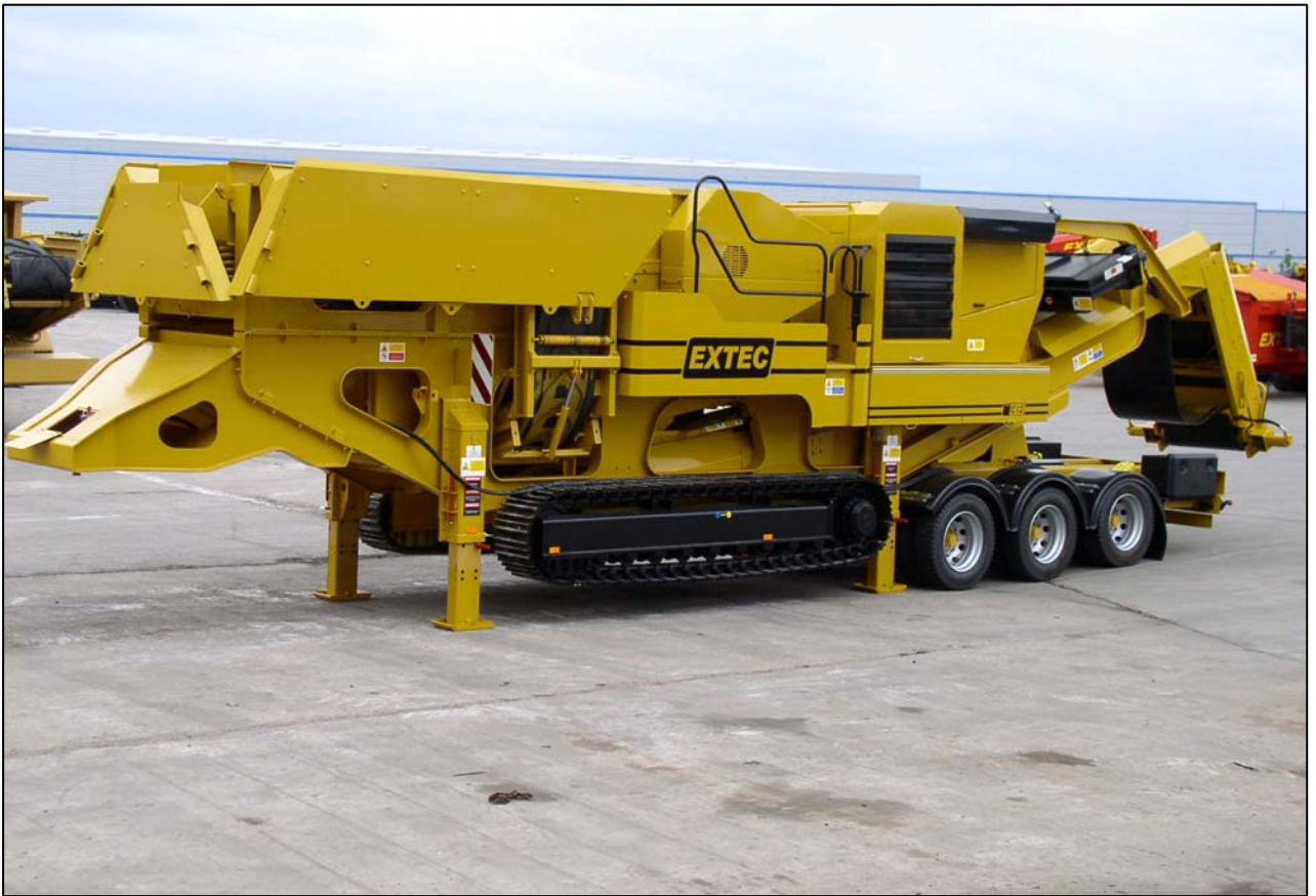
Optional bogie system – eliminates the need for low loader
