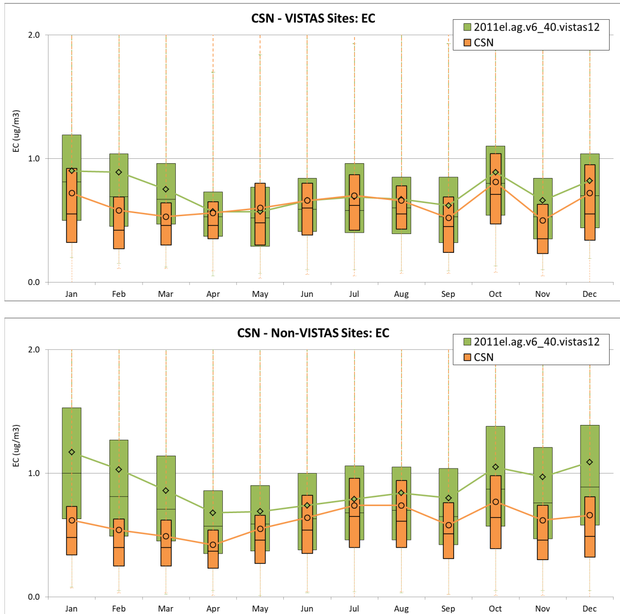
Figure 7-26. Boxplot Comparisons of Model Predictions and CSN Elemental Carbon (EC) Observations for Each Climate Region by Month.
