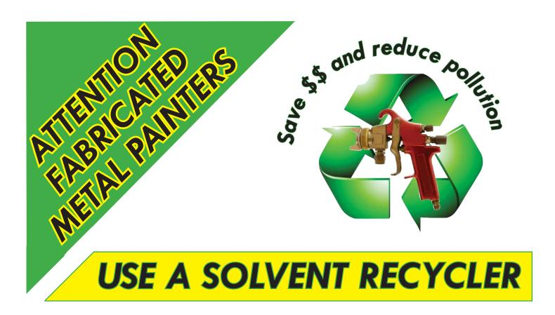
Instead of buying expensive solvent and having to dispose of spent solvent as hazardous waste, you can recover up to two-thirds of your spent solvent to use again with a solvent recycler.
