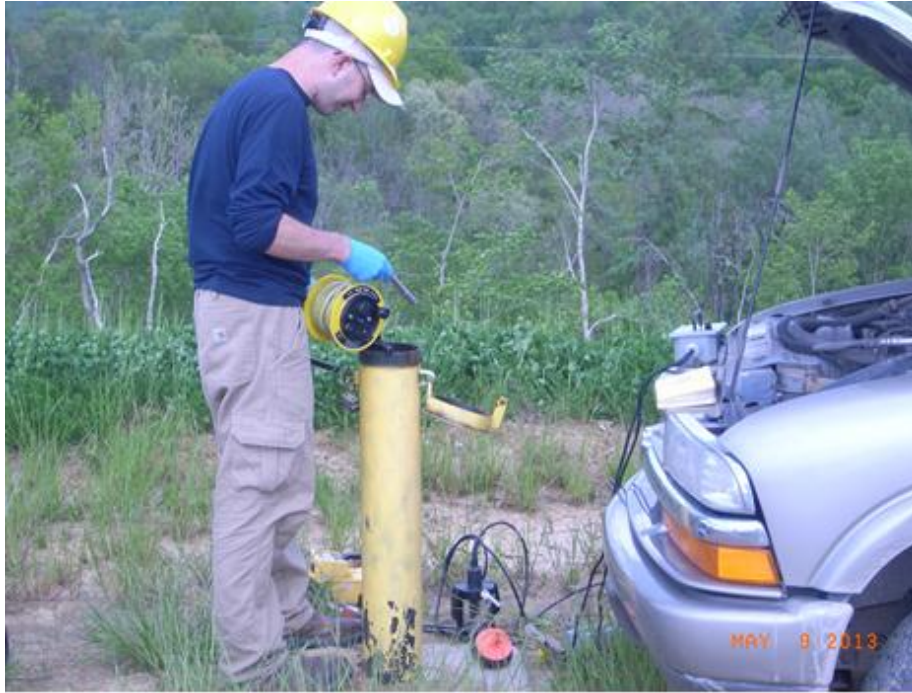
Figure 4: Measuring depth-to-bottom and depth-to-water at the SHL centralized pits site.
