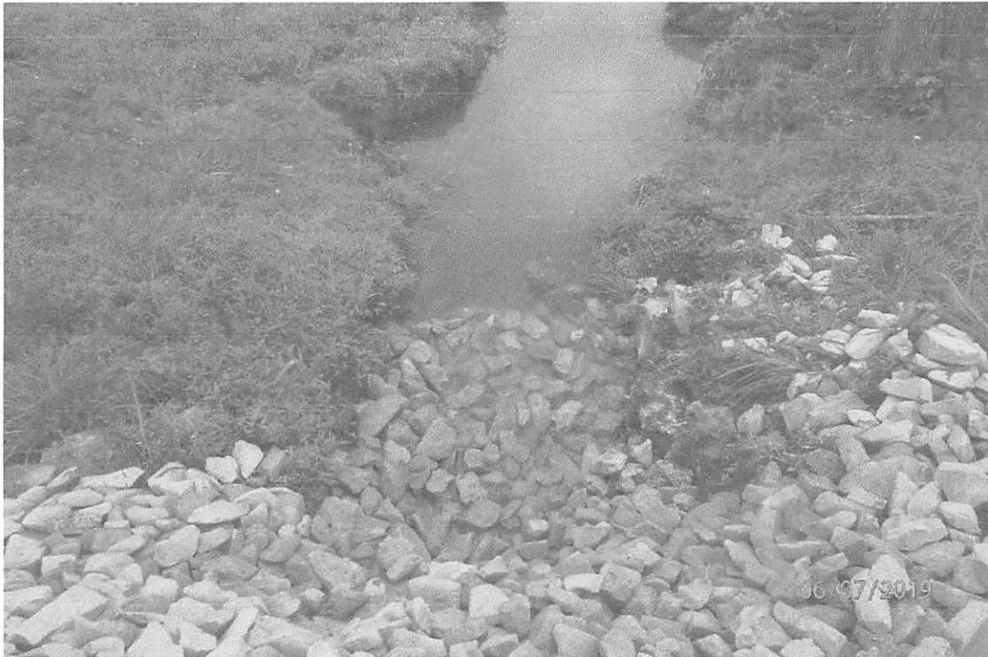
Stone that was placed in the stream by the site operator during the inspection at UNT Beards Run (39° 15.098' X 80° 10.735'). CNA deposits pictured downstream of the crossing.
