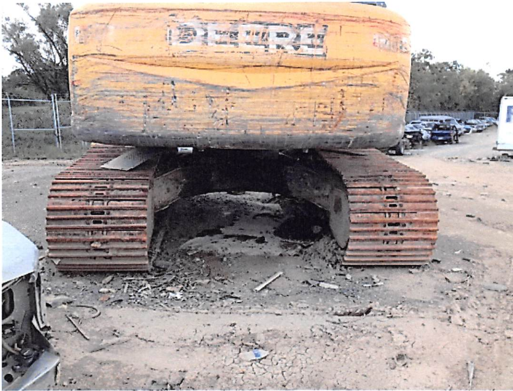
Spill with stay-dri under track excavator
