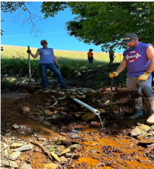
BRWA volunteers constructing a “flow-pipe” flow monitoring system for an acid mine drainage source in the Buckhannon River watershed.
