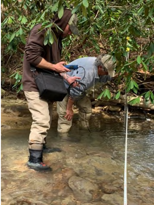
STTWA members measuring discharge on Beaver Creek.
