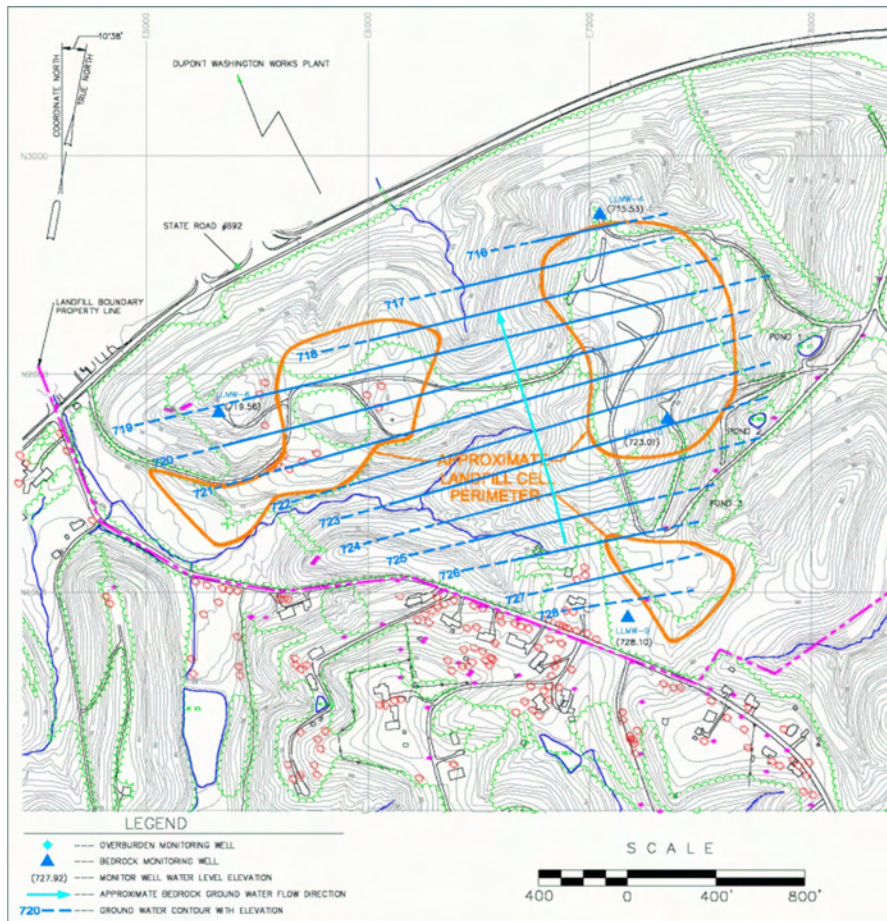
Figure 4.6: Local Landfill Zone A Top-of-Groundwater Map.
