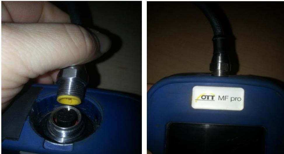
Figure 4-12. OTT MF Pro Cable attachment to Hand Set
