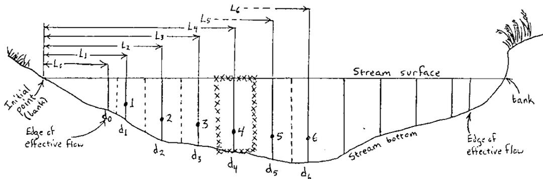
**Figure 4-1. Cross-Section Transect of a Stream Channel Divided into Subsections**
