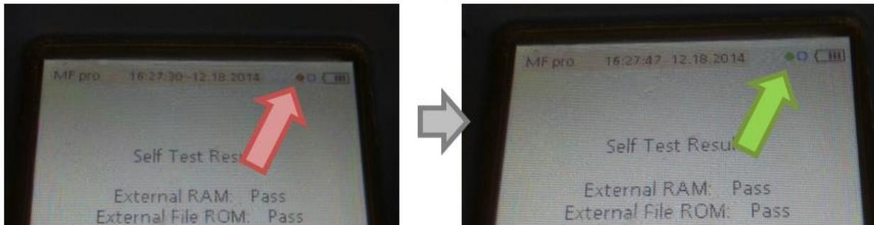
Figure 4-14. Red vs. Green Status Light on the OTT MF Pro Display Unit
