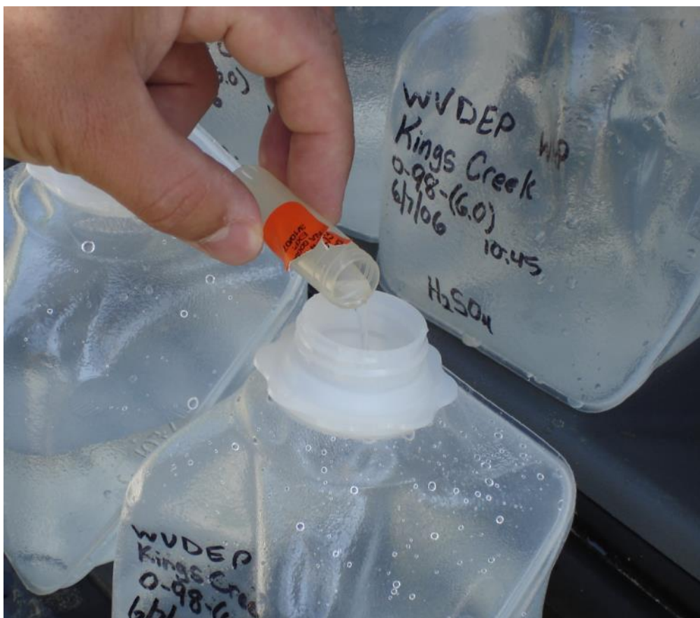
Figure 87. Example of sample being preserved with Nitric Acid.
