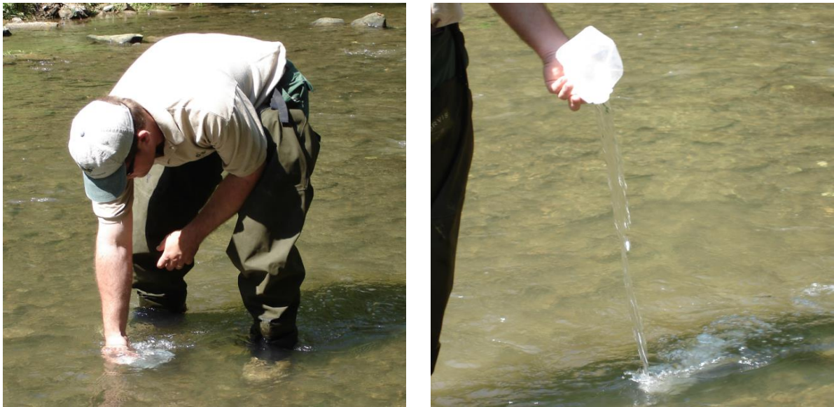
Figure 85. Example of Cubitainer being filled and emptied (i.e., rinsed with stream water).
