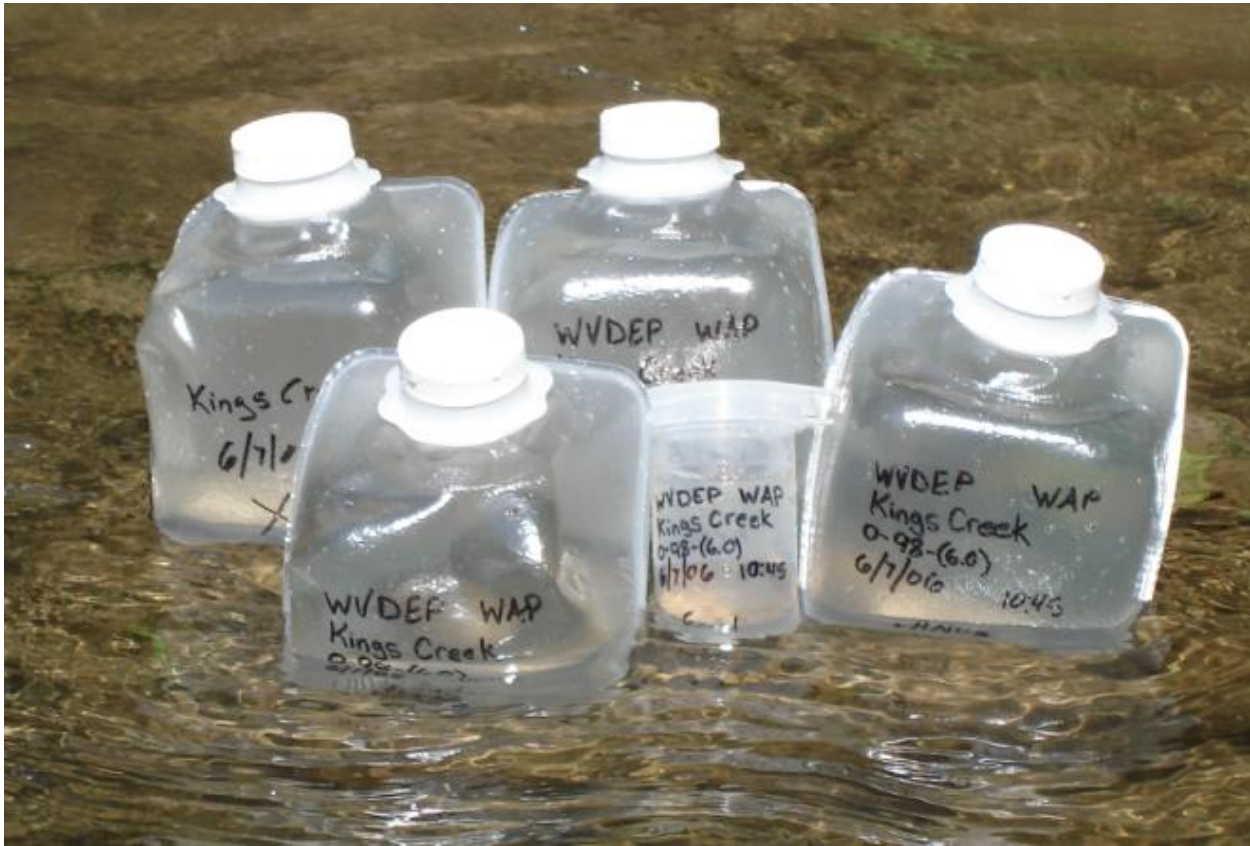
Figure 83. Example of Sample Containers Labeled with sample information.
