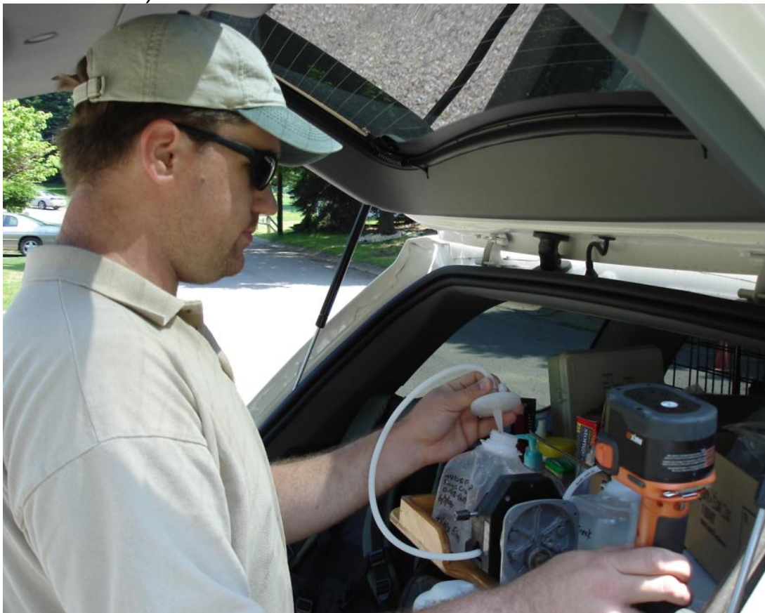
Figure 86. Example of Peristaltic Pump/Drill Apparatus for Sample Filtration being used under the tailgate of a vehicle.
