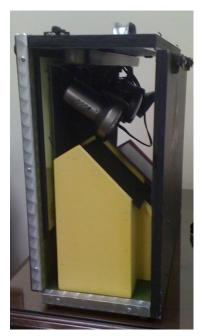
The display is constructed from 2 - 2'x 4' pieces of <sup>3</sup>/<sub>4</sub>" plywood. The wood was cut so that the display folds into a case for easy transport. It uses piano hinges at the joints and window latches to close the case and
