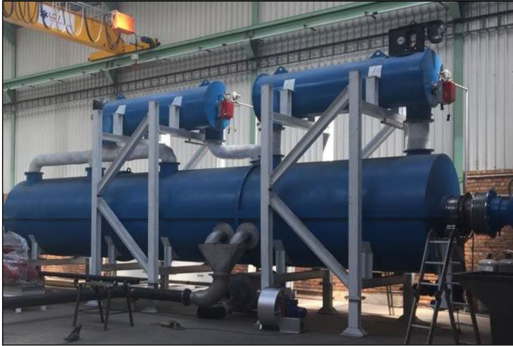
Figure 12. Photo of typical low temperature pyrolysis unit.
