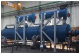
Figure 12. Photo of typical low temperature pyrolysis unit.
