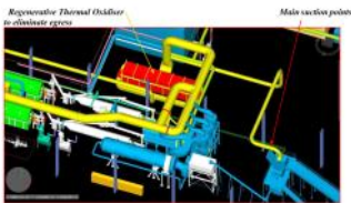
Figure 6. The Regenerative thermal oxidizer is maintained at 850°C.
