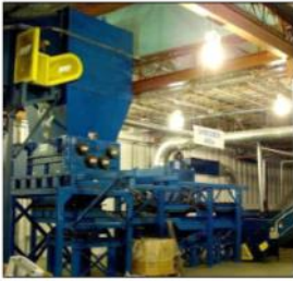
Figure 7. Photo of a typical Macerator/Grapple system.
