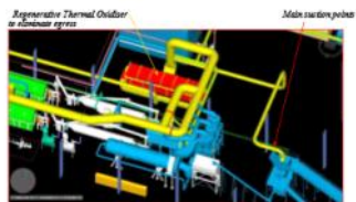
Figure 6: The Regenerative Thermal oxidiser is maintained at 1100°C
