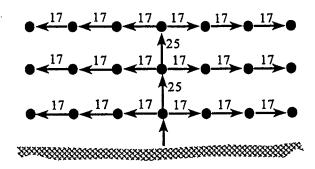
6. Study the sequential timer shot design below. Each hole contains 14 bags of ANFO each weighing 50 pounds and two water gel boosters. There are 22 water gel boosters to a case and a case weighs 55 pounds. The sequential timer is set for a delay of 33 milliseconds. Figure the
