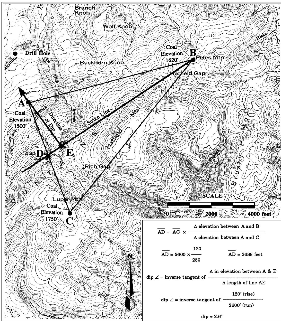
*Figure V-1.-Example of Strike and Dip Calculations Using a Three-Point Problem*
