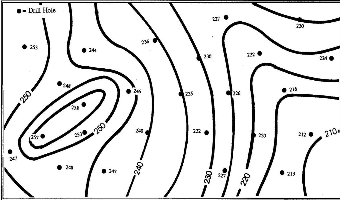
Figure V-10-a.—Isopach Map Showing Depth of Cover for an Underground Coal Mine
