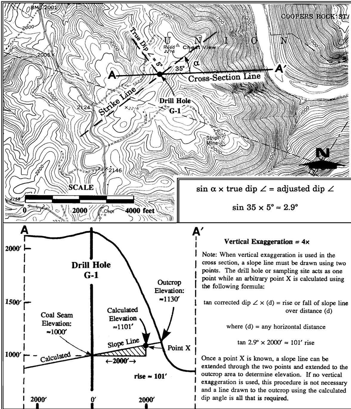
Figure V-2.-Example for Determination of Coal Outcrop Elevation
