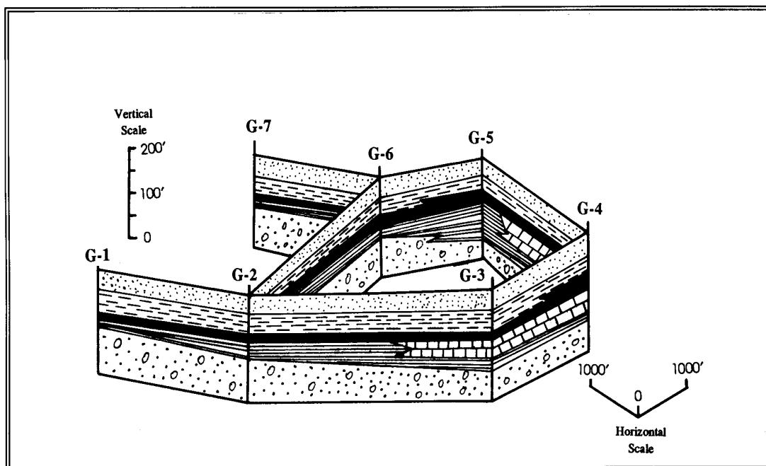
Figure V-7a.—Illustration of Fence Diagram
