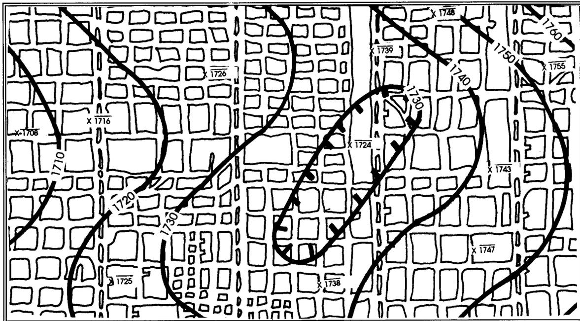
Figure V-9b.—Typical Structural-Contour Map Drawn Against And Underground Mine Workings Map
