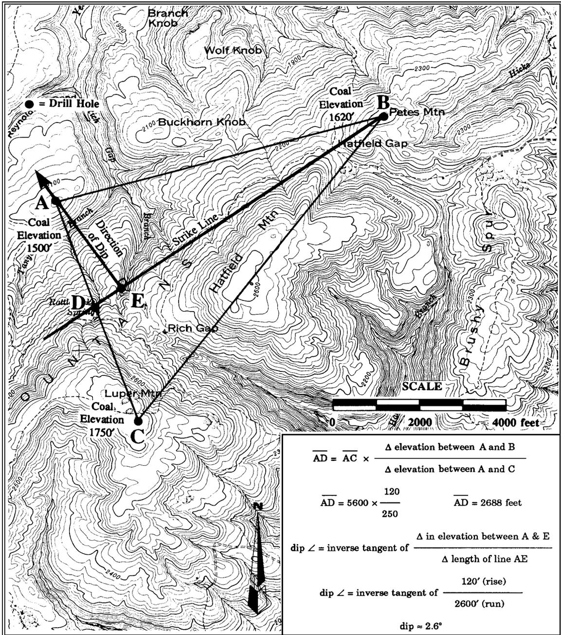
Figure V-1.-Example of Strike and Dip Calculations Using a Three-Point Problem
