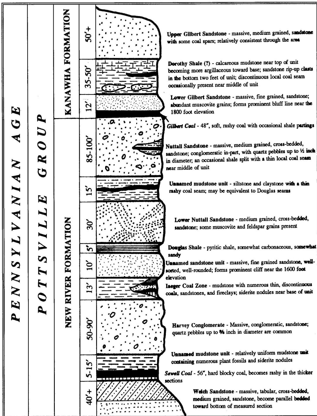
Figure V-6.-Composite Geologic or Stratigraphic Column
