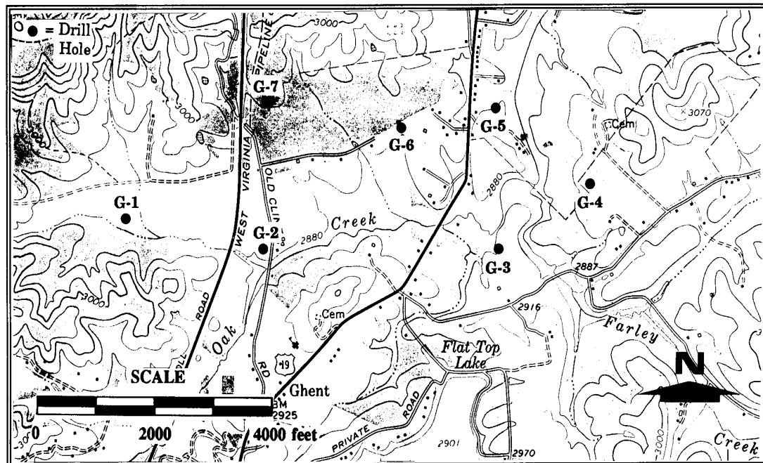
Figure V-7b - Locations and Relative Positions of Drill Holes
