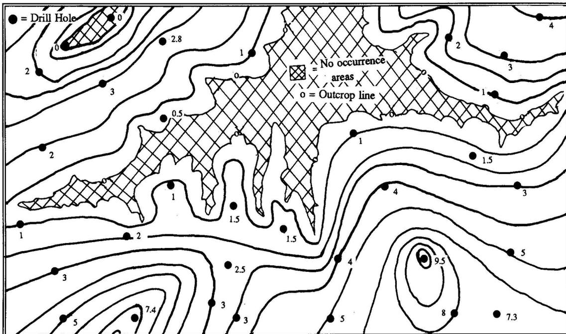
Figure V-10-b.—Isopach Map Showing the Relative Thickness of a Potentially Acid-Forming Shale Unit
