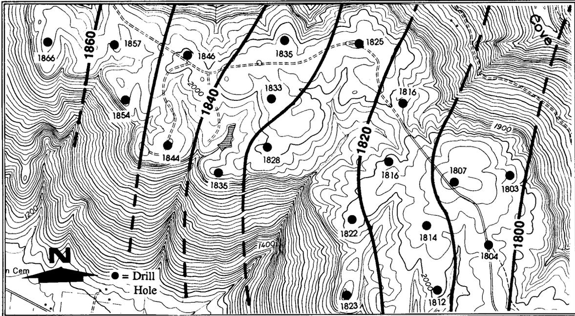
Figure V-9a.—Typical Structural-Contour Map Drawn on the Base of Coal Seam
