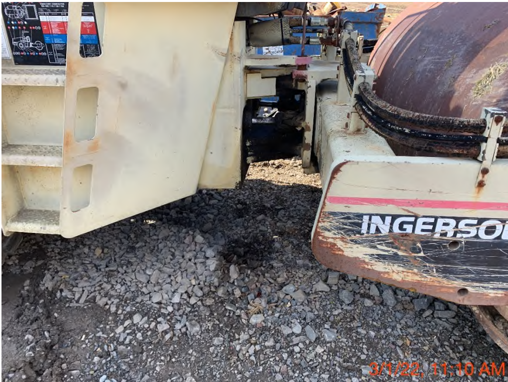
Equipment leaking onto ground
