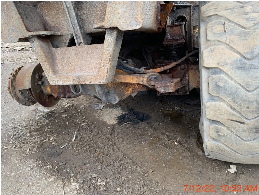
7/12/2022 Petroleum was leaking from a salvage truck onto the ground near the ditch.
