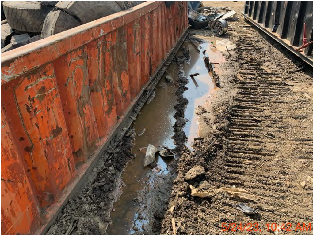
5/24/2023 There was petroleum staining on the ground around the scrap metal dumpster.
