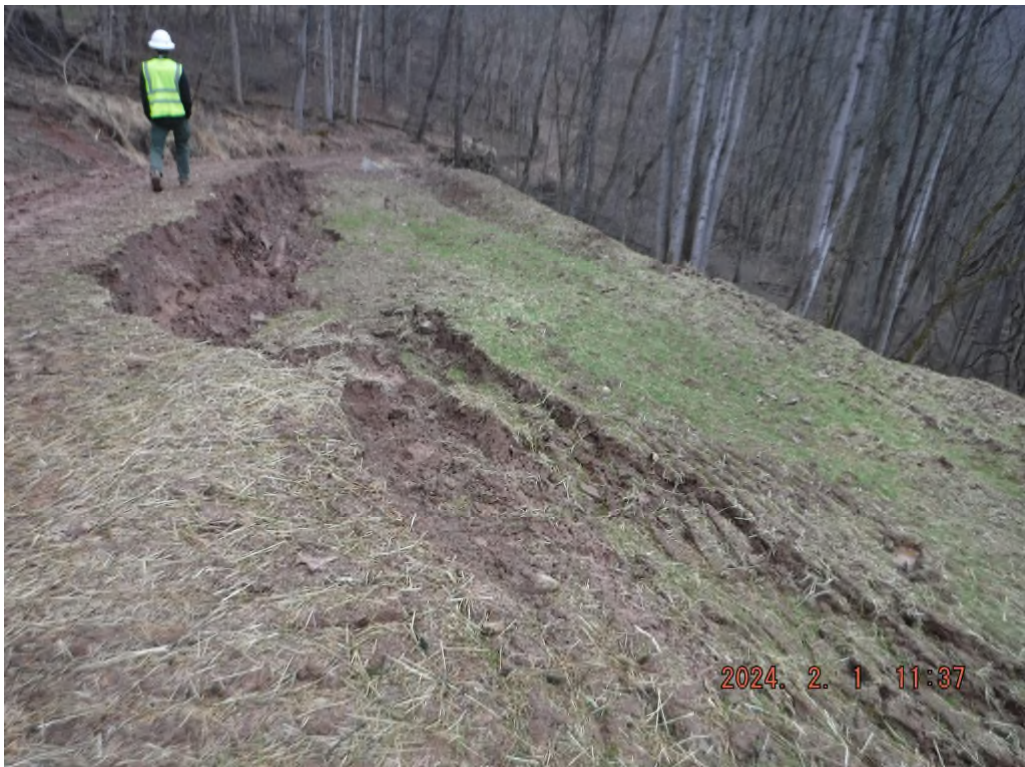
Photo # DSCF1620: Slip adjacent to the proposed access road on sheets 3 and 4.
