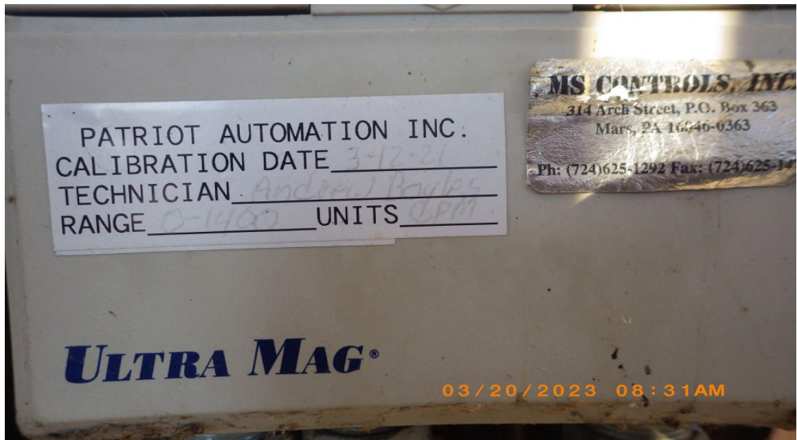
Flow Meter Calibration Sticker (date 3-12-21)
