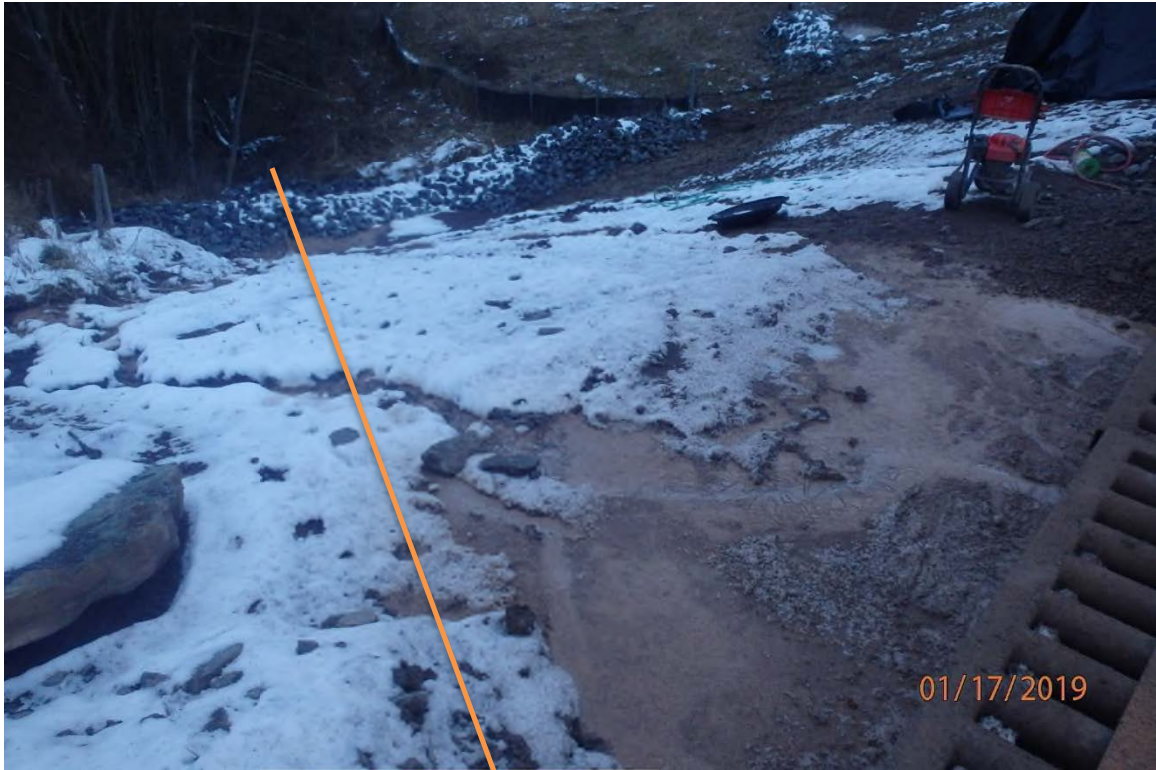
Area below truck wash showing path of sediment laden water.
