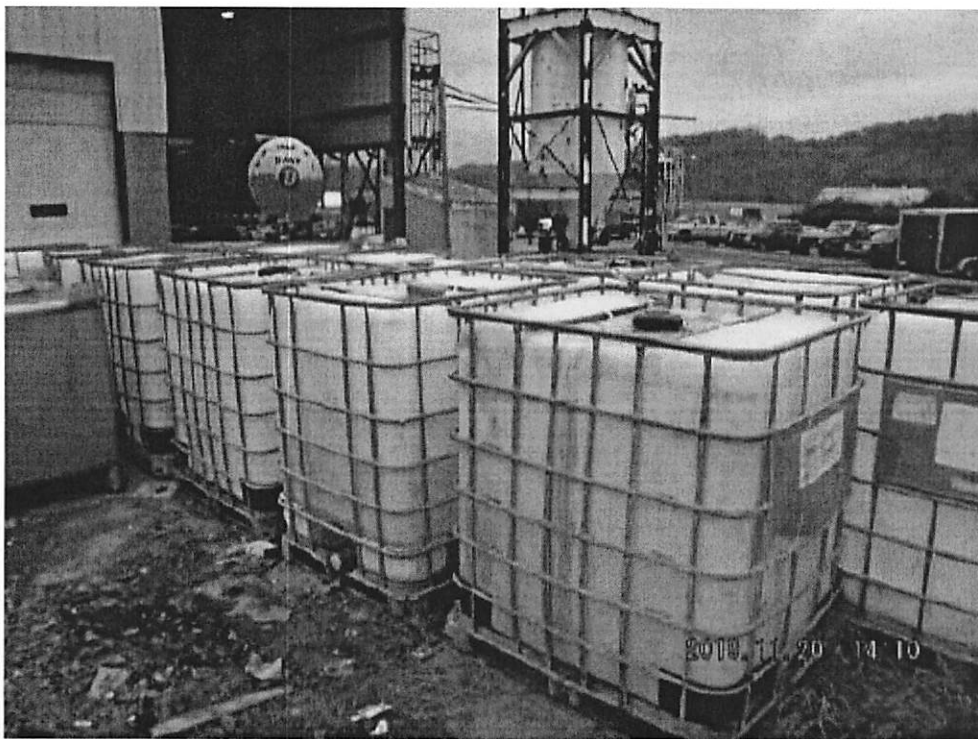
11.20.2019 – Chemicals stored without secondary containment.
