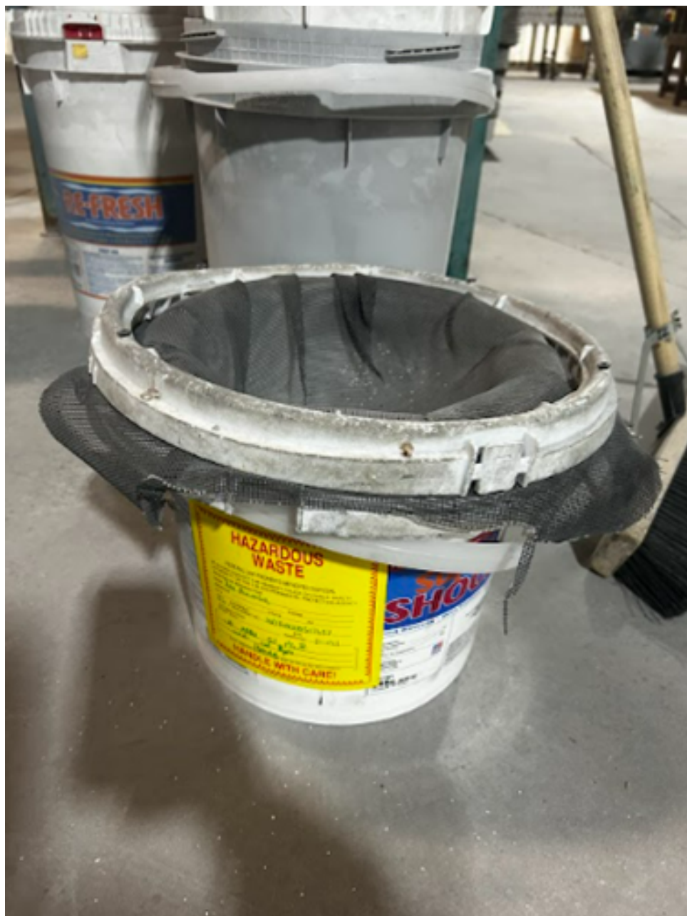
March 17, 2025 – A three-gallon plastic bucket of \text{Ca}(\text{OCl})_2 (calcium hypochlorite) floor sweepings properly labeled, but open.
