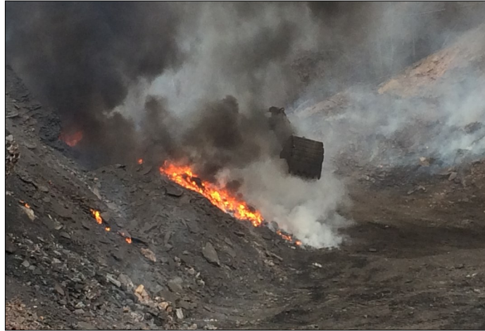
The basket of an excavator is barely visible among the smoke and flames rising from a burning coal refuse pile in Boone County. The burning material has to be spread out in order for it to cool enough to be moved.
