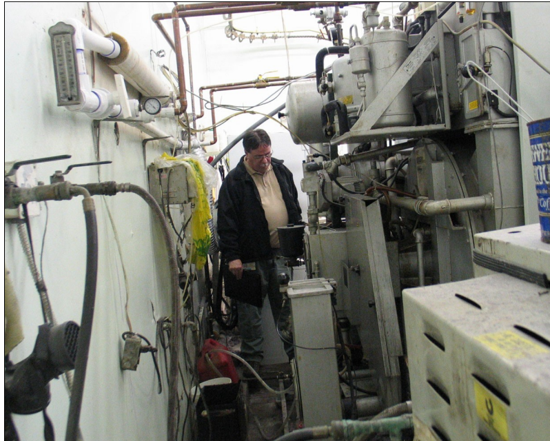
Top, Fred Teel, an inspector with the Division of Air Quality, looks over dry cleaning equipment at Mound Cleaners in South Charleston. Teel's focus is on potential leaks of perc, the toxic solvent used in the cleaning process. Right, Teel and owner Steve Krebs discuss information in the cleaner's log books.
