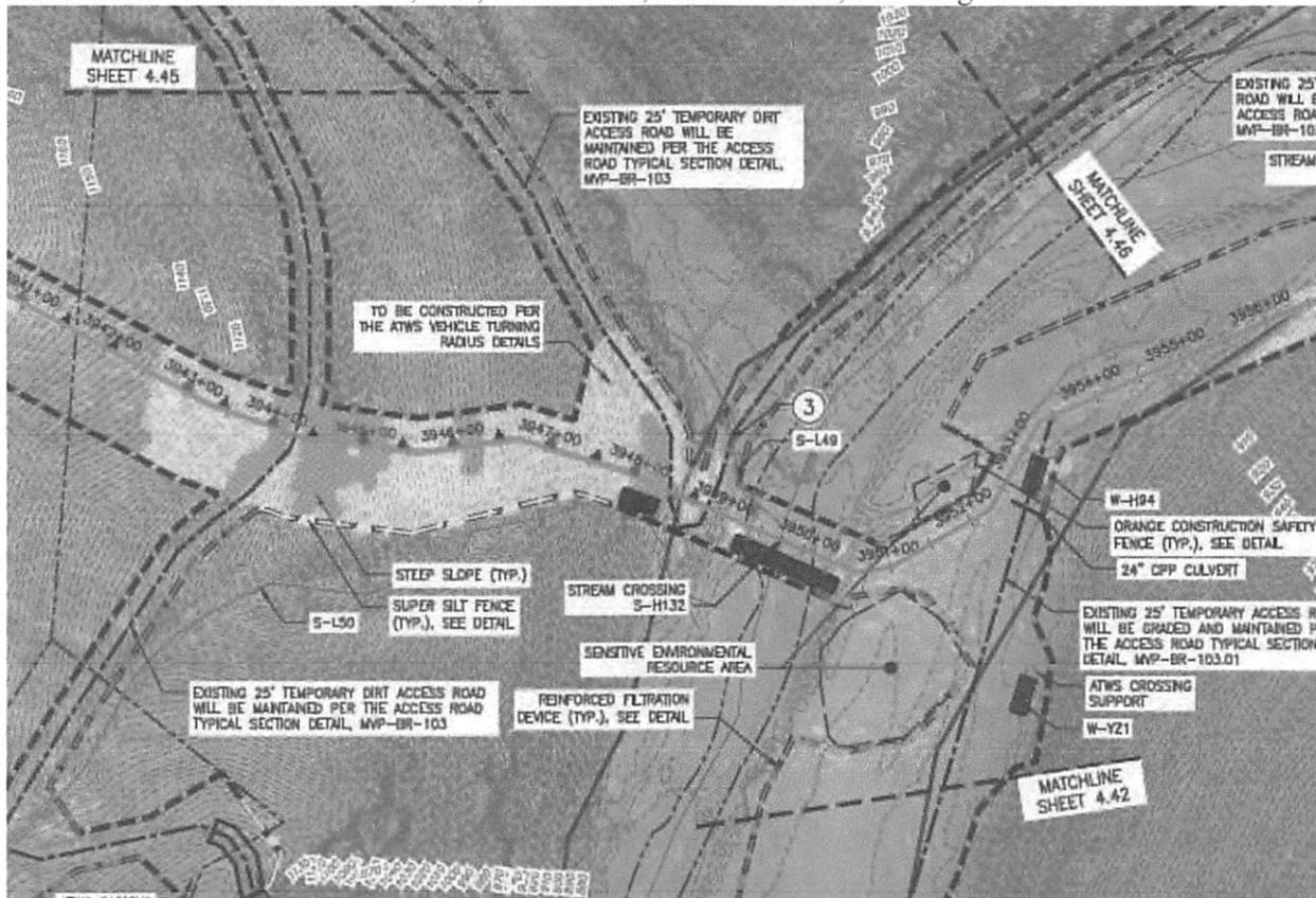
Approximate location of slip that impacted Elliott Run upstream of AR-MVP-BR-103 crossing with Elliott Run and downstream of where AR-MVP-BR-103 leaves MVP ROW upslope of Little Kanawha River crossing.
