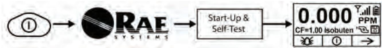
The instrument is now operating and performs self tests. If any tests (including sensor and memory tests fail), refer to the Troubleshooting section of the User's Guide.
