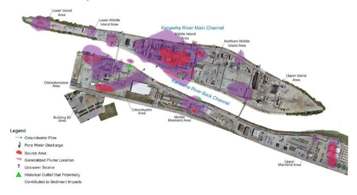
Figure 2.1 Revised Conceptual Site Model for Groundwater Discharges and Three Historic Outfalls (Jacobs 2020).
